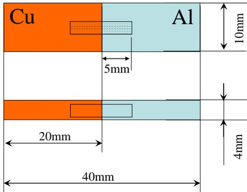
Fig. 5 Schematic diagram of joint sample of Cu/Al with carbon fiber.
