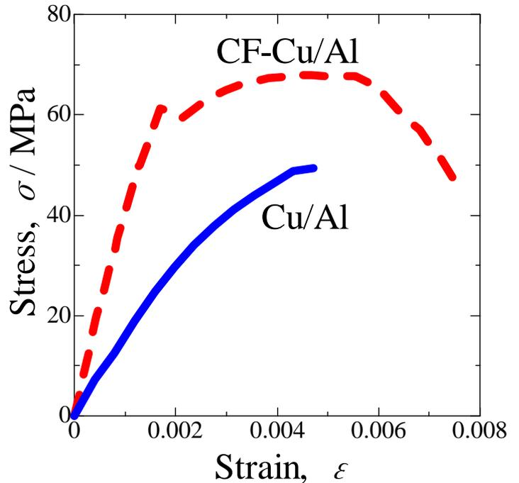
Fig. 6 Stress-strain curves of Cu/Al junctions with and without carbon fiber.
