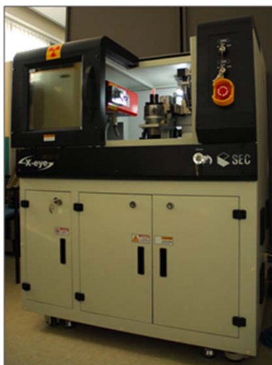
Fig. 2 Micro X-ray CT equipments of KICT
