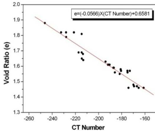
Fig. 6 Relation between void ratio and CT Number
