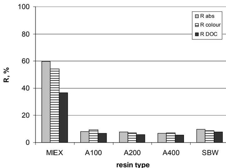
Fig. 2 Influence of resin type on NOM removal
