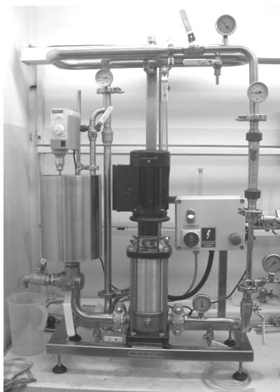
Fig. 1 Ultrafiltration cross-flow system
