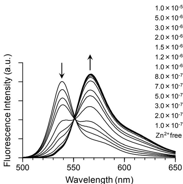
Fig. 2 Changes in the fluorescence spectrum of BDP-TPY with  $Zn^{2+}$ . The spectra are for  $Zn^{2+}$  concentrations of 0, 0.1, 0.2, 0.3, 0.5, 0.7, 0.8, 1.0, 1.2, 1.5, 2.0, 3.0, 5.0, and 10.0  $\mu M$ . Spectra were acquired in aqueous acetonitrile solution with excitation at 535 nm. The concentration of BDP-TPY was 1  $\mu M$ .
