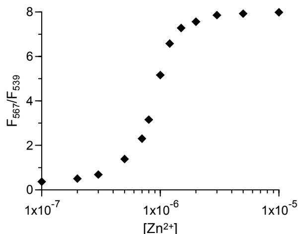
Fig. 3 Plot of the fluorescence intensity ratio (F<sub>567</sub>/F<sub>539</sub>) of BDP-TPY versus increasing Zn<sup>2+</sup> concentration.
