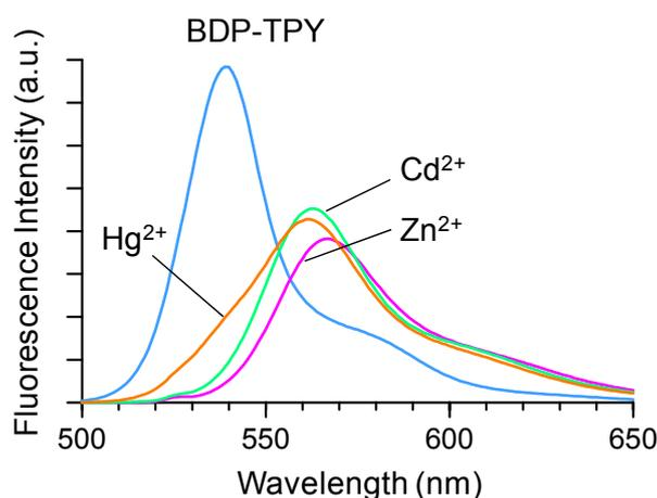
Fig. 1 Fluorescence spectra of BDP-TPY in the absence and presence of different metal ions (50  $\mu\text{M}$ ) in aqueous acetonitrile solution with excitation at 525 nm. The concentration of BDP-TPY was 1  $\mu\text{M}$ .
