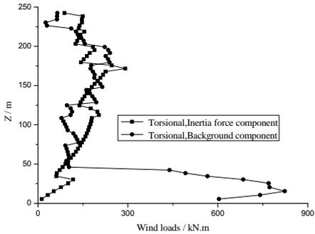
**Fig. 8** Comparison of Inertia force Item and quasi-static force Item equivalent wind loads in torsional direction under 0° wind azimuth
