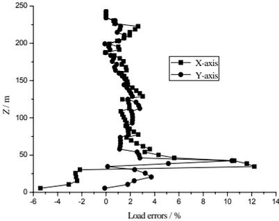
**Fig. 9** Deviation between the shearing force and bending moment equivalent wind loads under 0° wind azimuth
