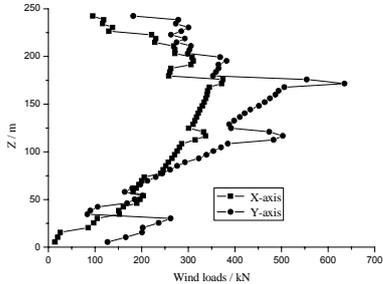
**Fig. 11** Equivalent wind load along X Axis and Y Axis under 90° wind azimuth
