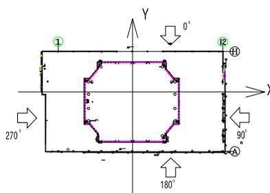
Fig. 5 Testing wind azimuths
