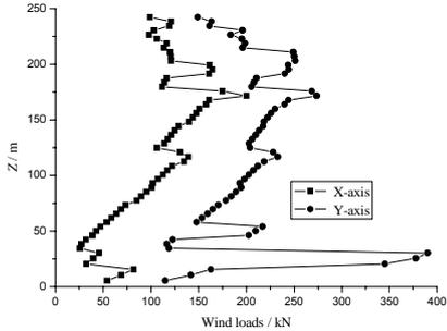
**Fig. 10** Equivalent wind load along X Axis and Y Axis under 0° wind azimuth
