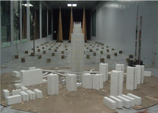
Fig.1 Model in wind tunnel
