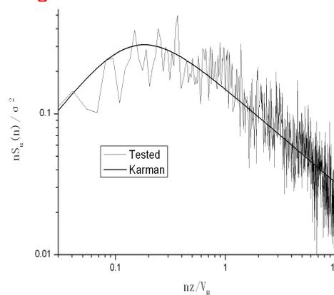
Fig. 4 Normalized wind speed spectrum
