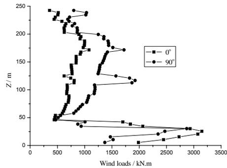
Fig. 12 Equivalent wind Load in torsional direction
