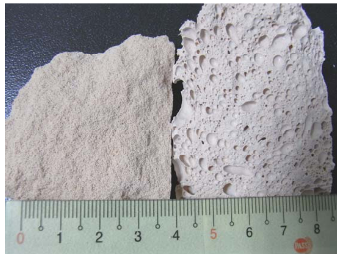
Fig. 2 the macrostructure of the metal powders foamed geopolymer (the right side) and the modifier-added foamed geopolymer (the left side)
