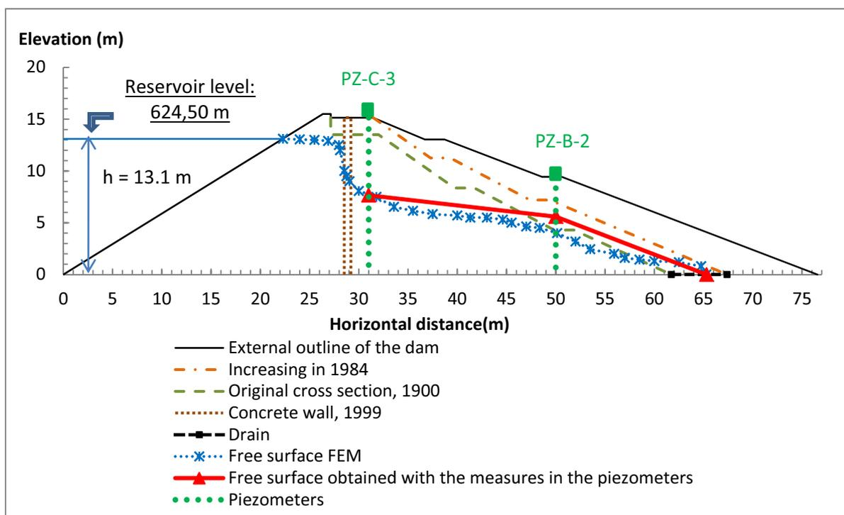
Fig. 6. Free surface position under steady conditions in the Gasset dam. Comparison between the real field piezometric levels and the numerical results obtained in the present research (free surface FEM).
