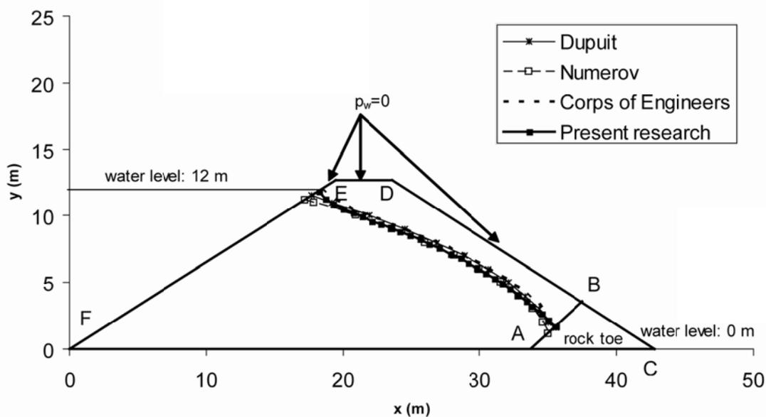
Fig. 2. Theoretical example of earth dam with available analytical solutions: homogeneous earth dam with a toe drain (Lambe and Whitman, 1979)
