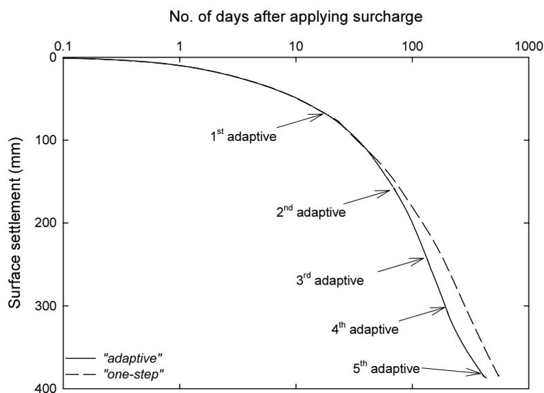
Fig. 3 Ground surface settlement profiles of *adaptive* and *one-step* analysis.
