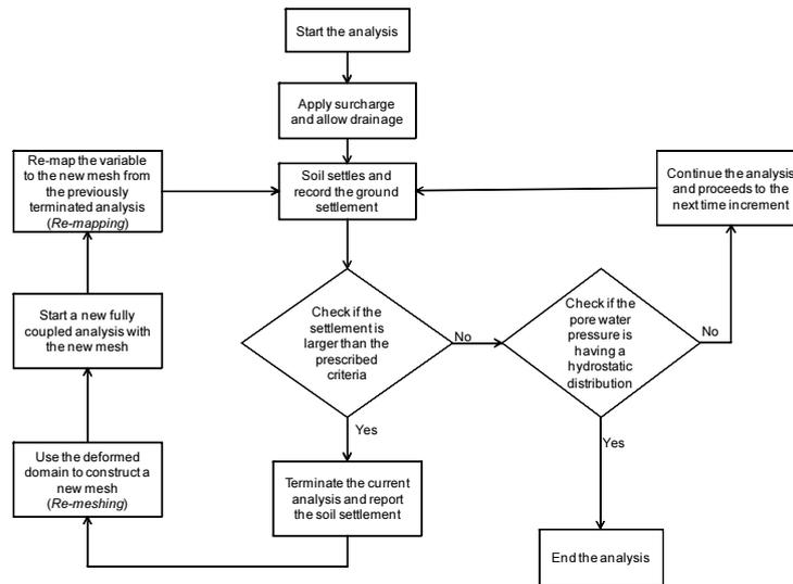
Fig. 2 Algorithm of the re-meshing and re-mapping process.
