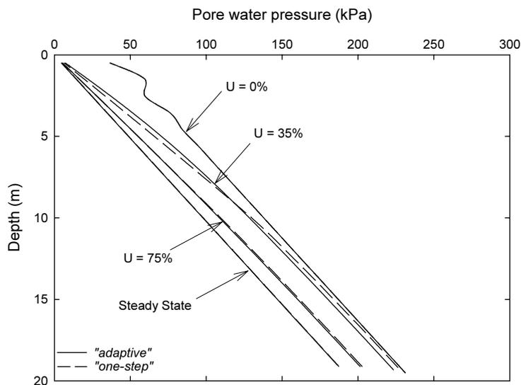
Fig. 4 Pore water pressure distribution of different analyses at different stages of the consolidation:  $U = 0\%$ ,  $U = 35\%$ ,  $U = 75\%$ , steady state.
