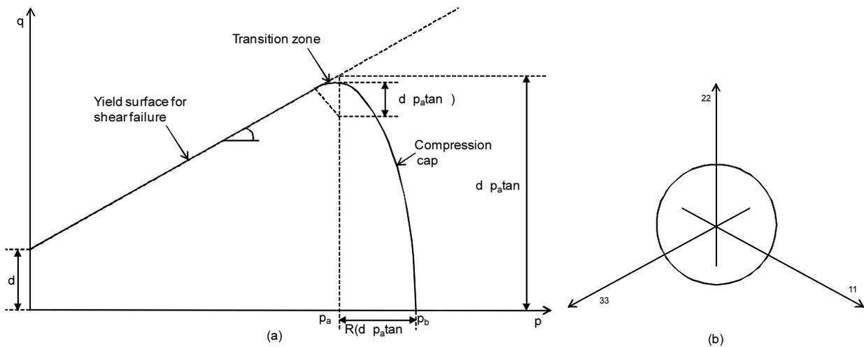
Fig. 1 Yield surface in (a) p-q plane, (b)  $\pi$ -plane.
