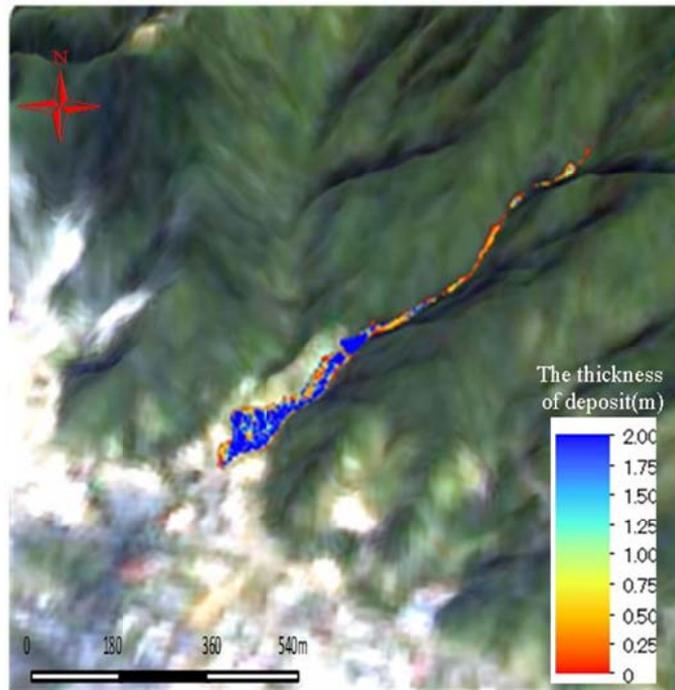
**Fig.9.** The thickness of deposit by fixed bed model
