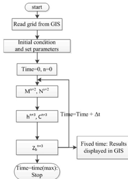
Fig. 4. The simple flow chart of the numerical simulation coupled with GIS.
