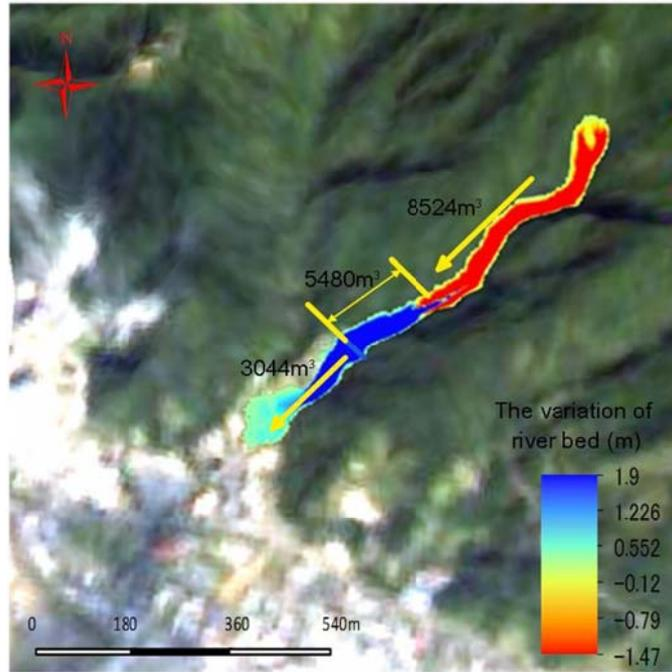
**Fig. 8.** The variation of river bed by mobile-bed model (T-model).
