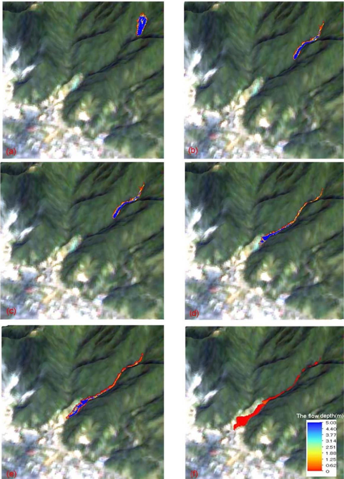
**Fig. 7.** The propagation and affected regions in different times ((a) 2s, (b) 40s, (c) 94s, (d) 110s, (e) 150s, (f) 220s).
