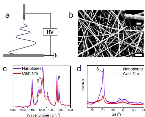
Fig. 1. a) Electrospinning setup, b) SEM images of electrospun PVDF nanofibers (scale bar: 2  $\mu\text{m}$ , inset scale bar: 200 nm). c) FTIR spectra of electrospun PVDF nanofibers and PVDF cast film. d) XRD patterns of electrospun PVDF nanofibers and PVDF cast film.
