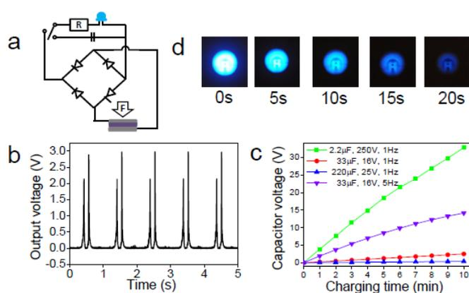
Fig. 3. a) Circuit for charging a capacitor and lighting a LED device, b) DC voltage output rectified from 1 Hz compressive impact of a  $16 \text{ cm}^2$  nanofiber membrane, c) voltage ~ charging time relationship for a nanofiber membrane device loaded with different capacitors, d) still frames captured from a video showing the continuous lighting of a blue LED.
