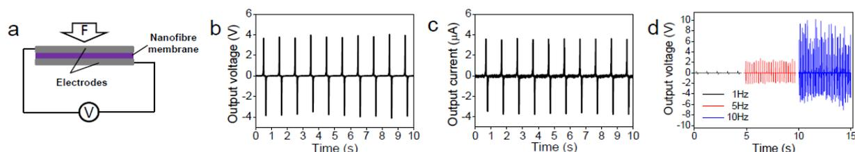
Fig. 2. a) Schematically illustration of the power generation device, b) voltage and c) current outputs of a nanofiber device under a 1 Hz compressive impact (working area,  $16 \text{ cm}^2$ ), d) relationship between impact frequency and the voltage output (working area,  $2 \text{ cm}^2$ )
