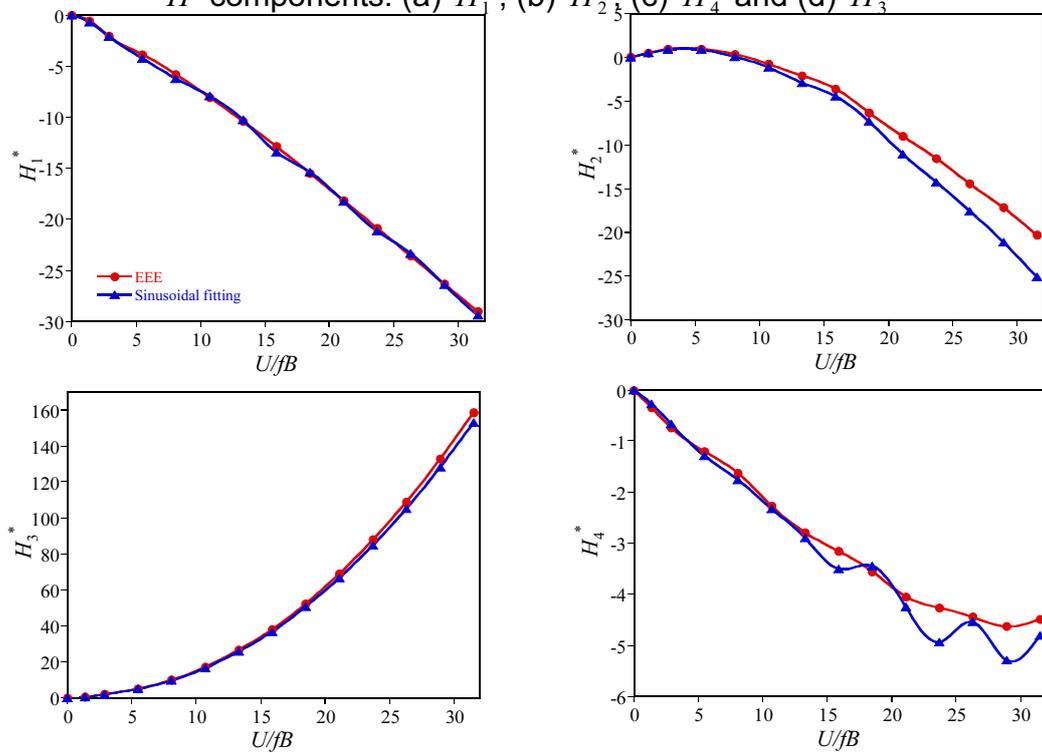
Fig. 2 Identified flutter derivatives from the forced vibration test for the B/D20 section -  $H^*$  components: (a)  $H_1^*$ , (b)  $H_2^*$ , (c)  $H_4^*$  and (d)  $H_3^*$
