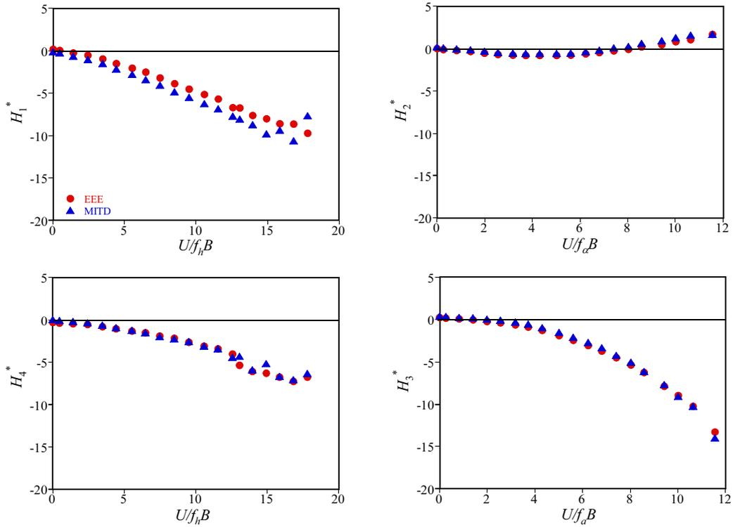
Fig. 1 Identified flutter derivatives from the free vibration test for the B/D20 section -  $H^*$  components: (a)  $H_1^*$ , (b)  $H_2^*$ , (c)  $H_4^*$  and (d)  $H_3^*$
