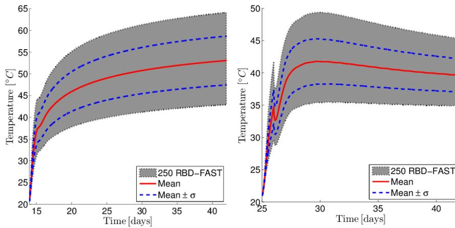
a) Point 1, in the center of the dam      b) Point 2, near the upstream face
