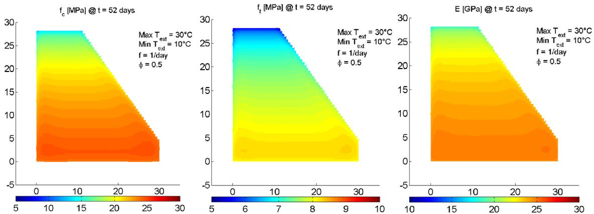
Fig.7 Properties' contours at the end of construction
