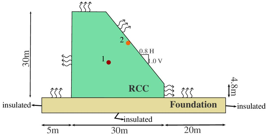
Fig.3 RCC dam model
