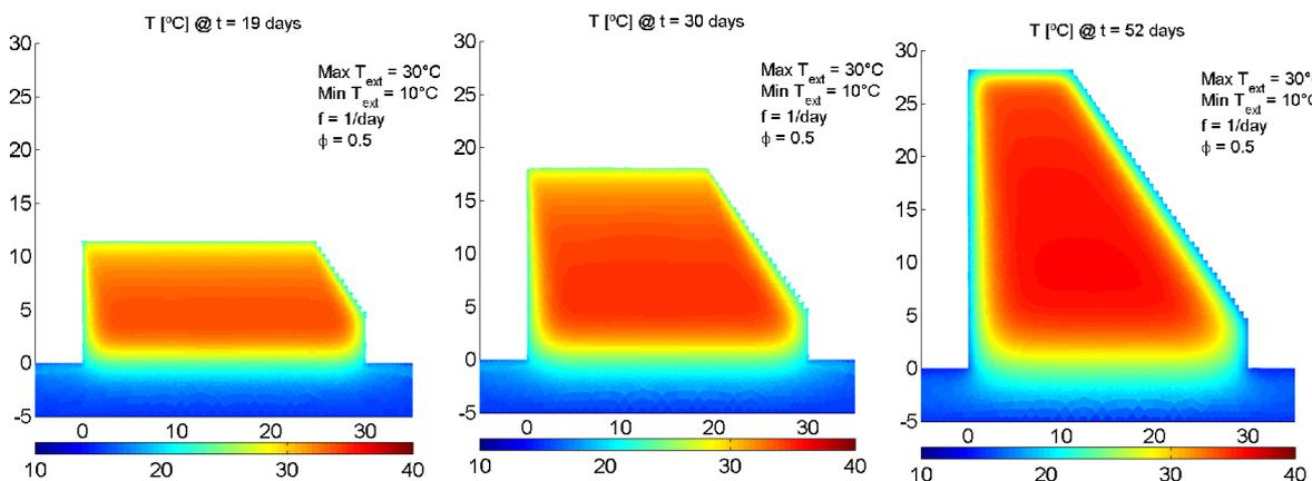
Fig.6 Temperature contours evolution during construction
