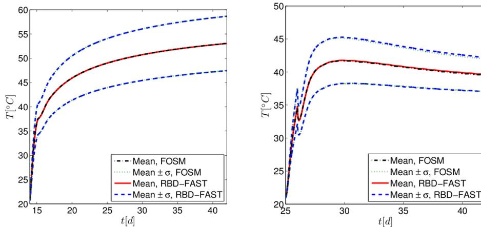
a) Point 1, in the center of the dam      b) Point 2, near the upstream face
