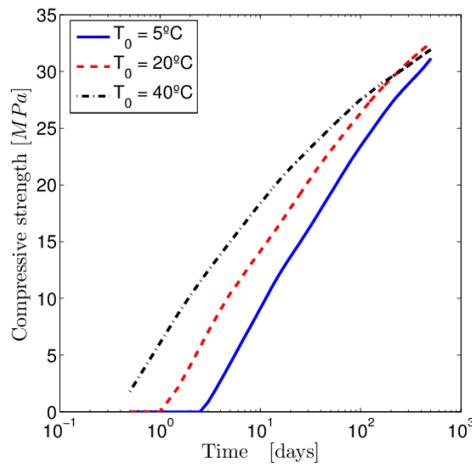
Fig.2 Compressive strength evolution, isothermal tests
