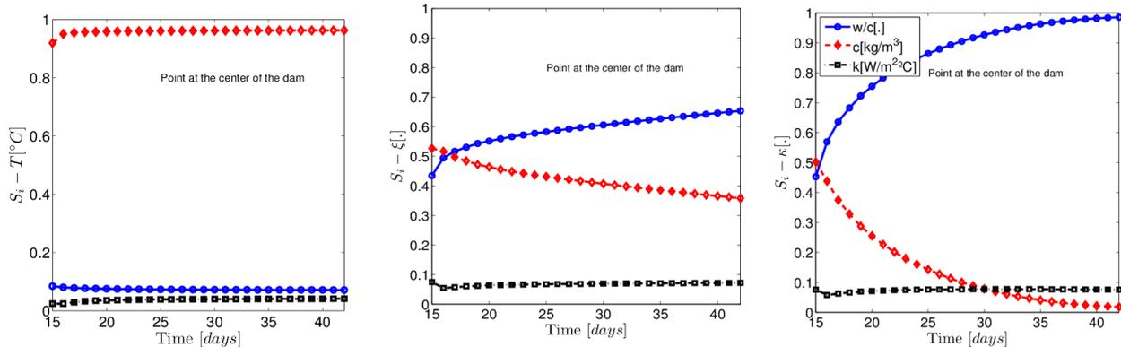
a)  $S_i$  for  $T [^{\circ}C]$ , point 1      b)  $S_i$  for  $\xi [.]$ , point 1      c)  $S_i$  for  $\kappa [.]$ , point 1
