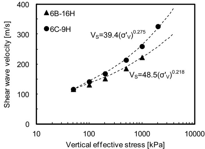
Fig. 3. Evolution of shear wave velocities during loading.
