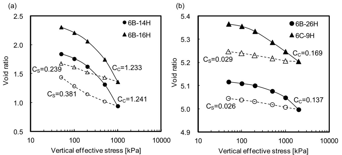
Fig. 2. Stress-volume response during loading (solid symbols) and unloading (empty symbols): (a) 6B-14H and 16H; (b) 6B-9H and 26H.
