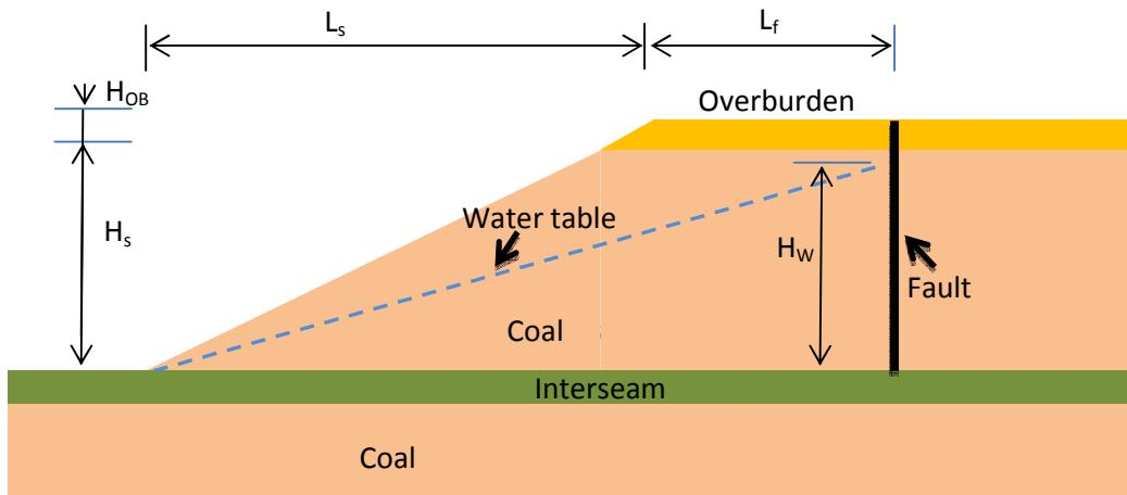
Fig. 1. A typical slope in brown coal open cut
