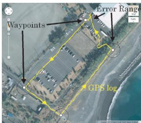
Fig. 14 Preliminary experiment in a coastal location (Image via Google Maps)
