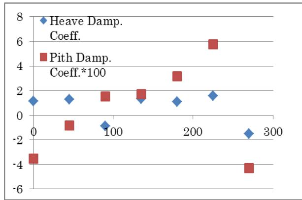
Fig. 21 Nondimensionalized heave and pitch damping coefficient of the foil combined motion. The foil section is NACA0015, depth / Chord = 0.33,  $\lambda$  / Chord = 2.6.
