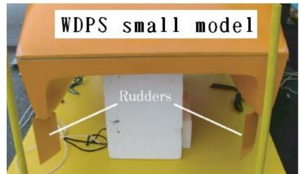
Fig. 6 Two rudders are installed to steer the WDPS vessel.
