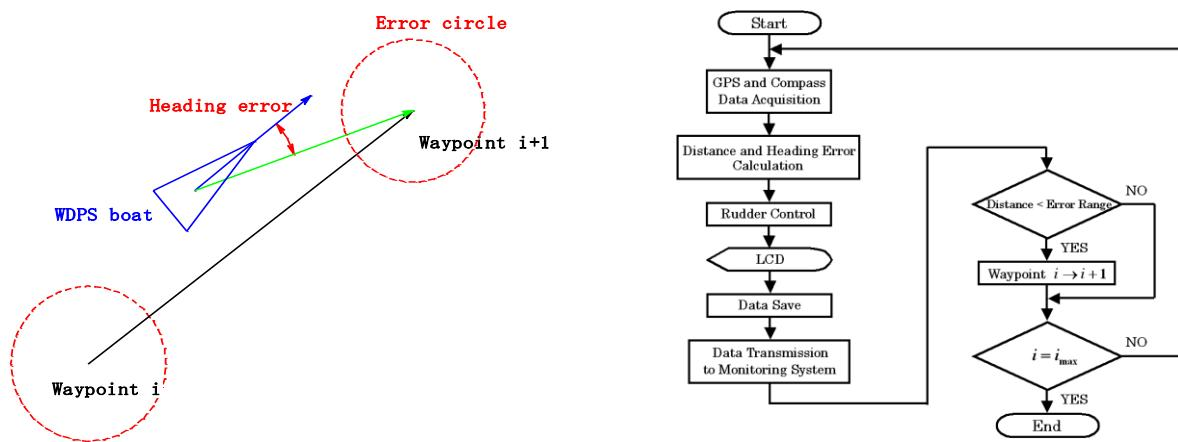
Fig. 10 Schematic view of waypoint and error circle
