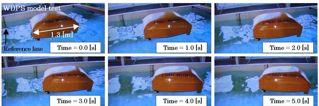
Fig. 7 WDPS wave tank test. Regular wave height is 0.1 [m]; wave length is 1.5 [m]. Advance speed against the waves is 0.16 [m/sec].
