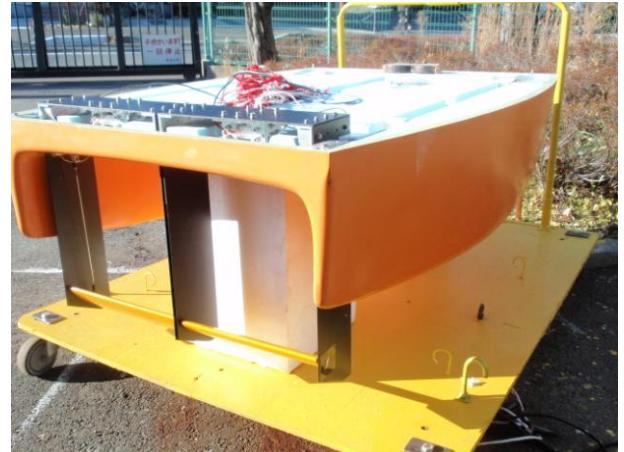
Fig. 4 Small newly designed dual fin type WDPS model. The upper cover is removed.
