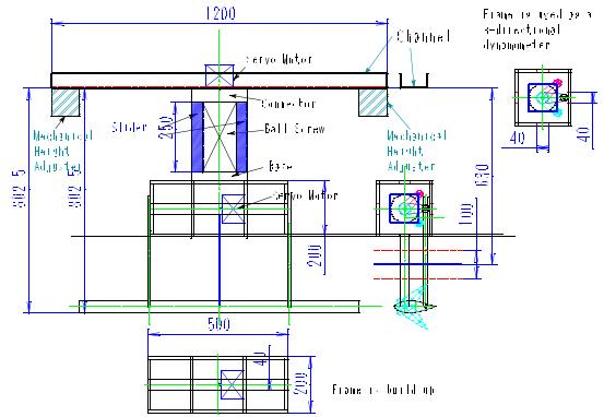
Fig. 20 Newly designed hydrofoil forced oscillator.
