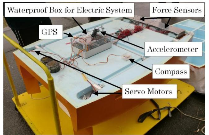
Fig. 15 Experimental setup for WDPS vessel sea trials.
