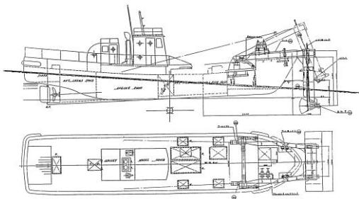
Fig. 2 Single fin type WDPS designed for actual sea trials (Terao 1990)
