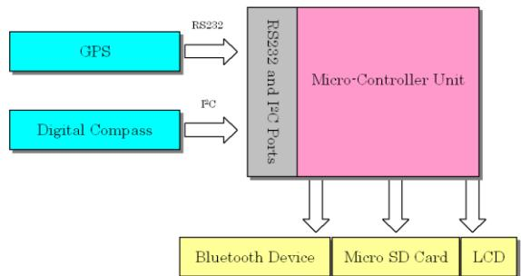
Fig. 9 Autonomous control system for the WDPS vessel
