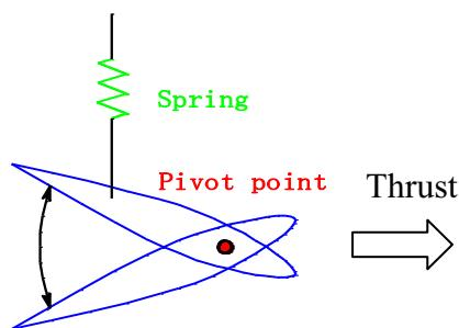
Fig. 5 Pitch restoring spring and fin pivot position. Hydrofoil oscillation generates thrust.
