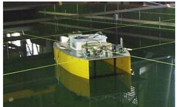
Fig. 3 Dual fin type WDPS testing in a wave tank (Terao 2000)
