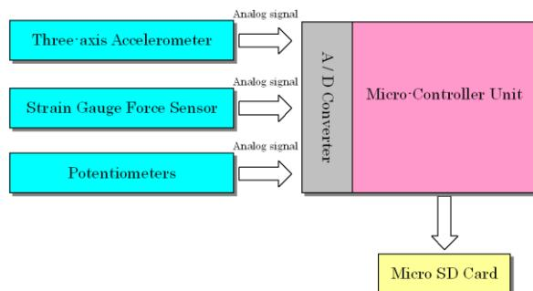
Fig. 8 Measurement system for the WDPS vessel
