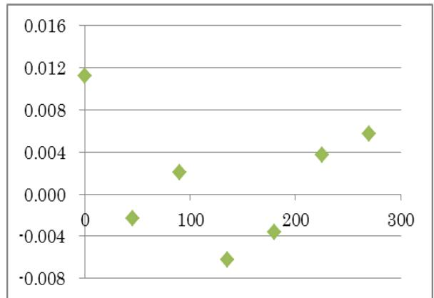
Fig. 22 Nondimensionalized steady surge force under the foil combined motion. The foil section is NACA0015, depth / Chord = 0.33,  $\lambda$  / Chord = 2.6.
