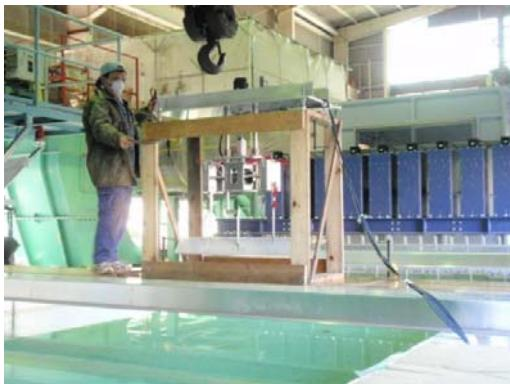
Fig. 19 Newly developed hydrofoil forced oscillator undergoing wave tank testing.
