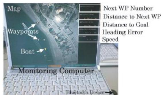
Fig. 13 Computer monitor displaying vessel progress and state
