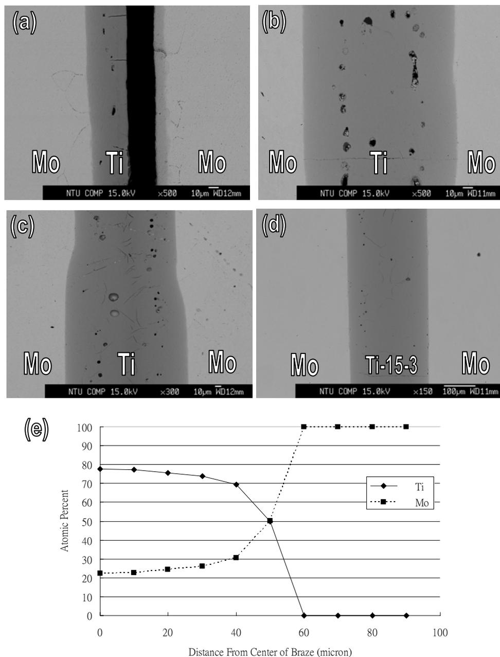
**Fig. 2.** EPMA BEIs and WDS analysis results of (a) Mo/Ti(40 μm)/Mo joint brazed at 1953 K for 600 s, (b) Mo/Ti(120 μm)/Mo joint brazed at 1983 K for 600 s, (c) Mo/Ti(160 μm)/Mo joint brazed at 2013 K for 600 s, (d) Mo/Ti-15-3(400 μm)/Mo joint brazed at 1903 K for 600 s, (e) WDS analyses across the joint of (b).
