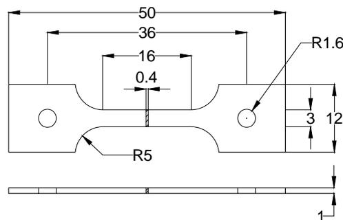
**Fig. 1.** Schematic diagram of tensile test specimen
