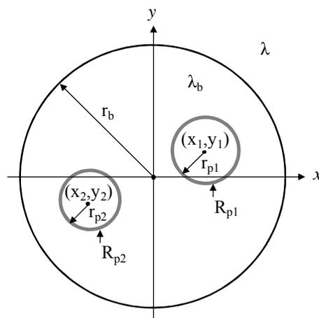
Fig. 1. Multipole method for two pipes in a borehole.
