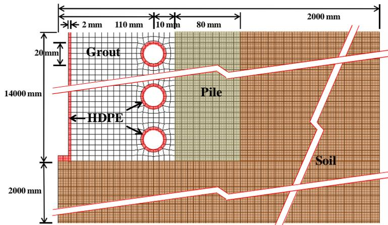
Fig. 2. Schematic view of numerical simulation.
