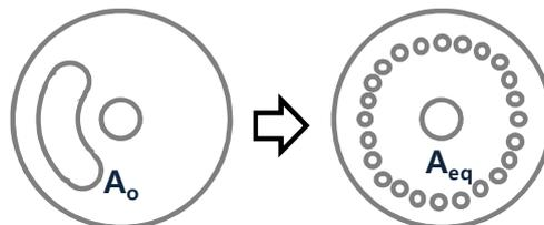
Fig. 4. Cutting face A-A' of spiral coil GHE.
