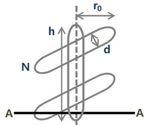
Fig. 3. Side view of spiral coil GHE.
