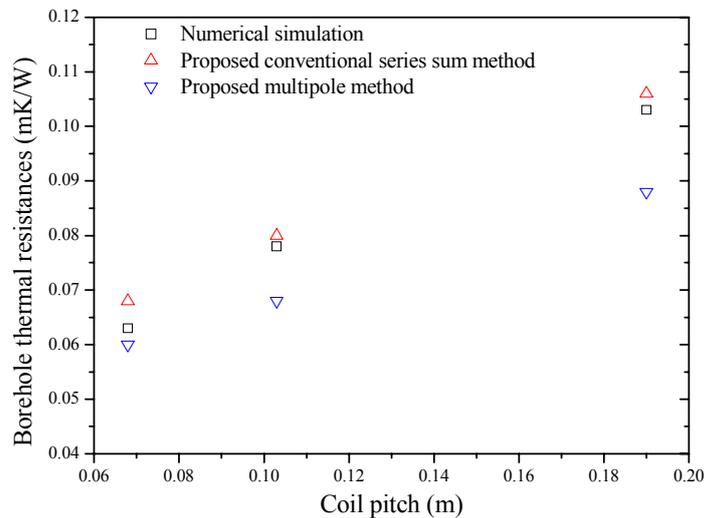
Fig. 5. Thermal resistances of borehole for spiral coil GHE.
