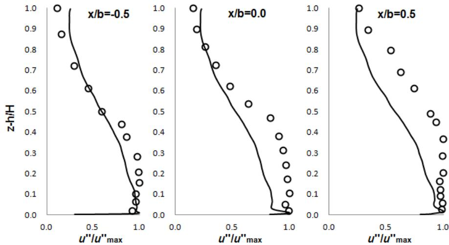
Fig. 10 Vertical profile of the ensemble average streamwise velocity fluctuations  $u''/u''_{\max}$ . —: LES results and o : current experimental results
