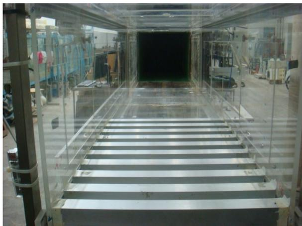
Fig.3. Arrangement of roughness elements in test section
