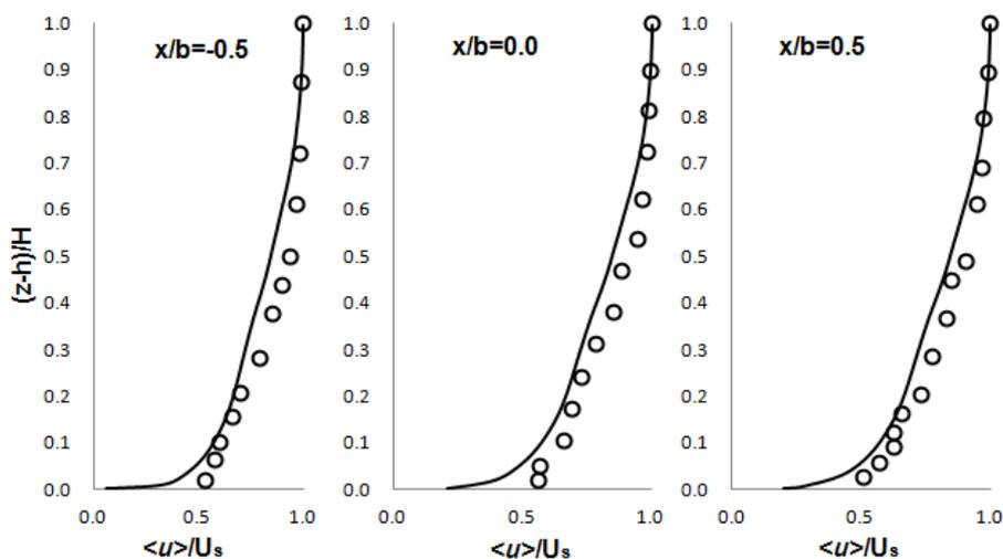
Fig.8. Vertical profile of the ensemble average streamwise velocity  $\langle u \rangle / U_s$ .
