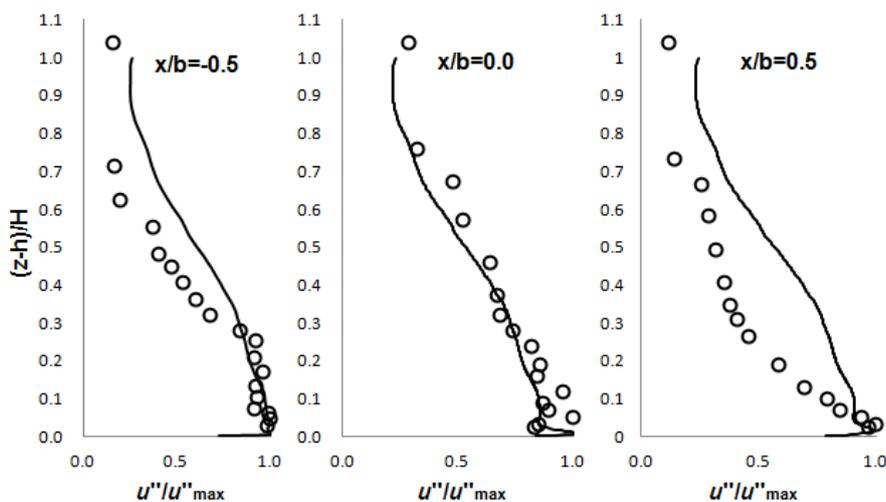
Fig.7. Vertical profile of the ensemble average streamwise velocity fluctuations  $u''/u''_{max}$ .
