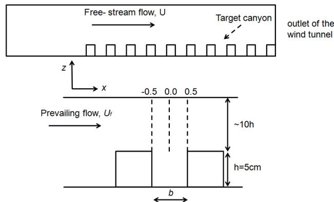
Fig.5. Schematic diagram of a detailed view of the sampling street canyon
