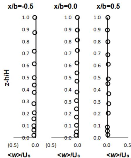
Fig.9. Vertical profile of the ensemble average vertical velocity  $\langle w \rangle / U_s$ .
