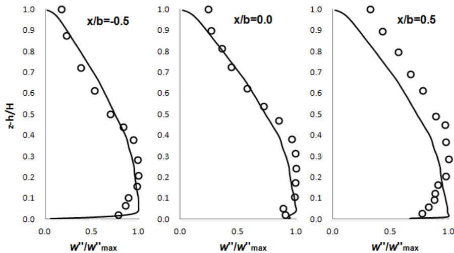
Fig. 11 Vertical profile of the ensemble average vertical velocity fluctuations  $w''/w''_{\max}$ . —: LES results and o : current experimental results
