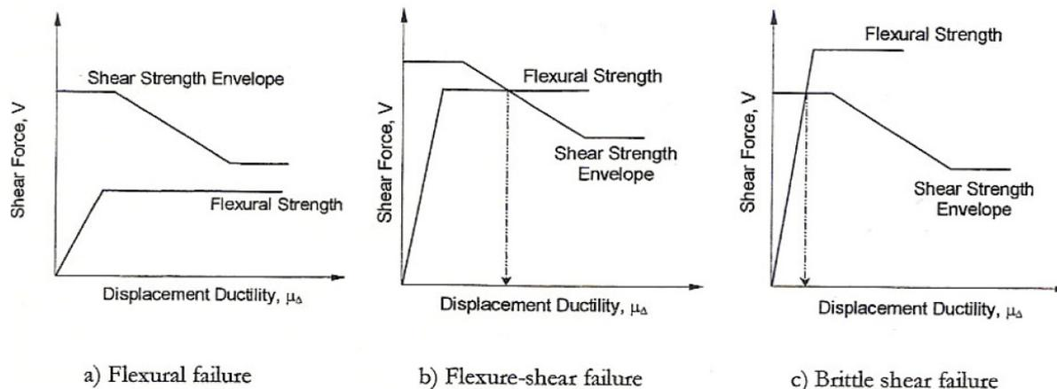
Fig. 5. Coupling Beam Failure Modes (Miranda et al., 2005)
