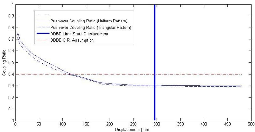
Fig. 8. Coupling ratio vs. top displacement
