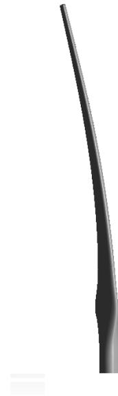
Fig. 9 Deformed blade shape exaggerated by 20 times
