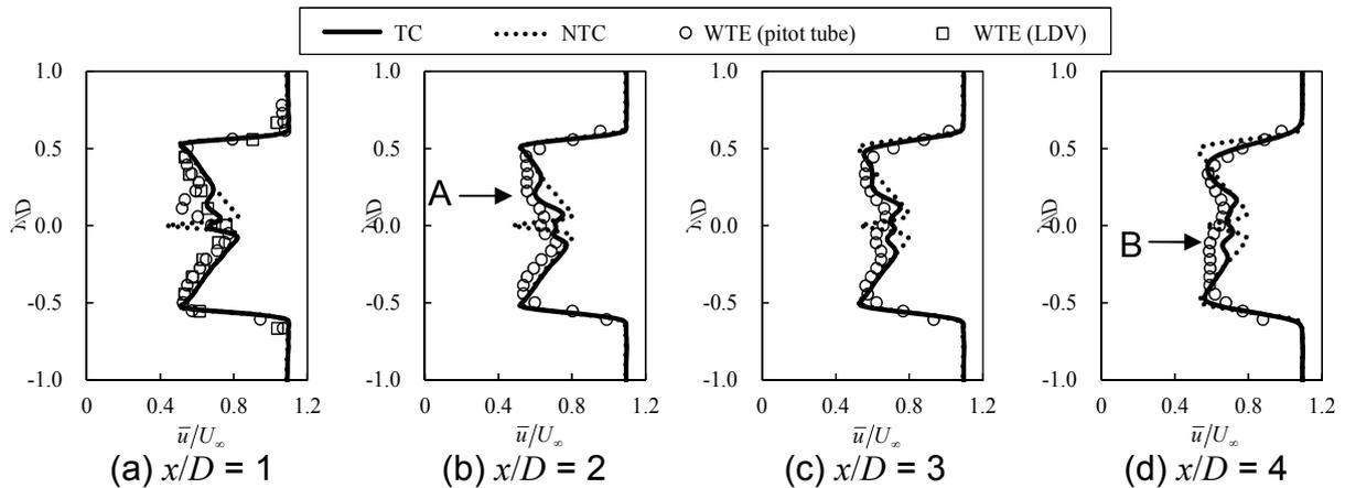
Fig.8 Spanwise distribution of the streamwise wind velocity at the hub height in the wind turbine wake. “WTE” represents the wind-tunnel experiments from Krogstad and Adaramola (2011).
