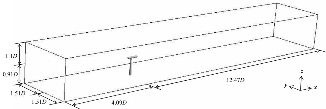
Fig.2 Computational domain ( $D$ : rotor diameter, 0.894 m)
