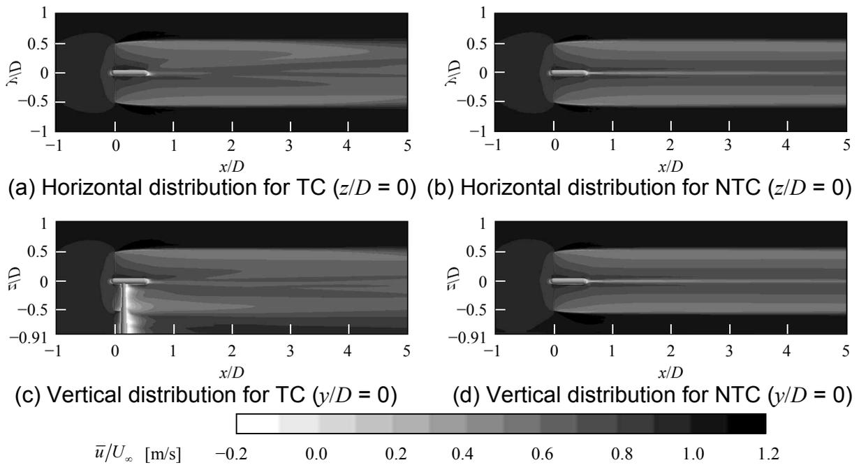
Fig.10 Contour plots of the time-averaged streamwise wind velocity (horizontal and vertical cross-sections through the rotor center)
