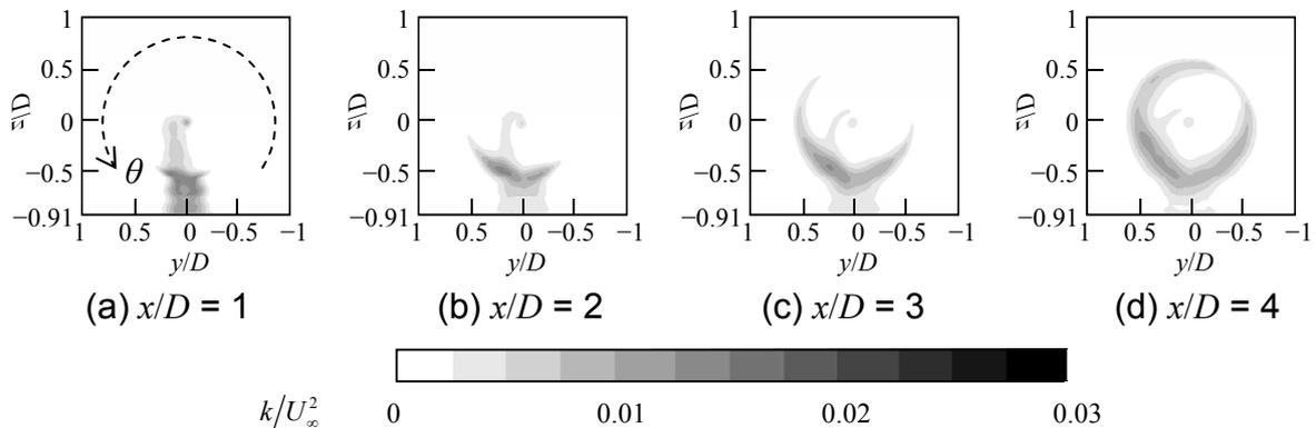
Fig.12 Contour plots of turbulence kinetic energy ( $y$ - $z$  cross sections at  $x/D = 1 - 4$  in TC)
