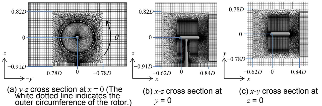
Fig.3 Computational grids in the vicinity of the wind turbine (origin: rotor center)
