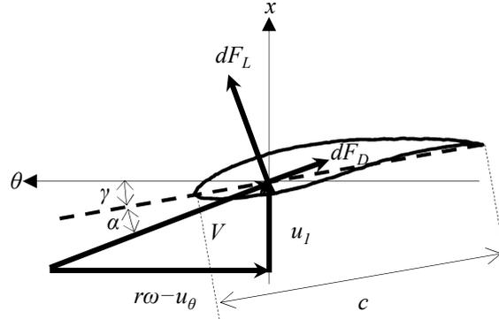
Fig.1 Relationship among the relative wind velocity,  $V$ , the lift,  $dF_L$ , and the drag,  $dF_D$ , acting on a blade element.
