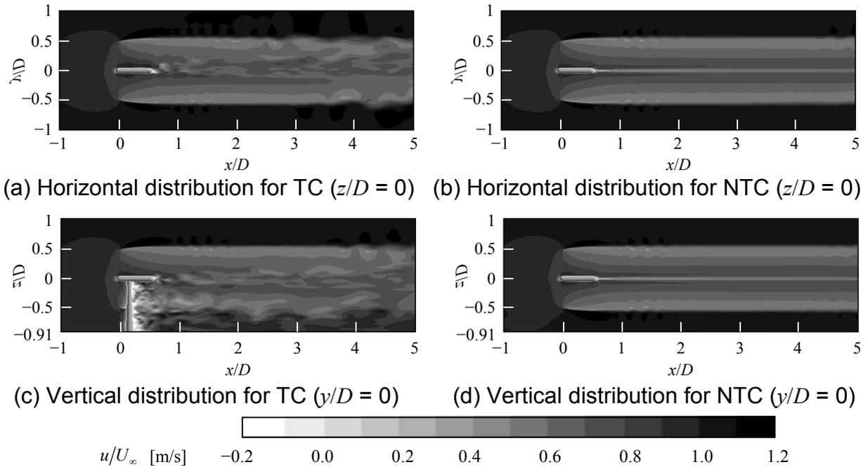
Fig.9 Contour plots of the instantaneous streamwise wind velocity (horizontal and vertical cross-sections through the rotor center)
