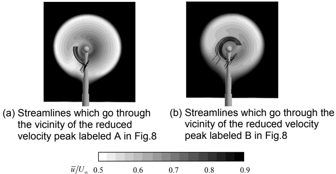
Fig.13 Streamlines of the time-averaged flow field (The  $y$ - $z$  cross-sections of the velocity field for peaks A and B are those from  $x/D = 2$  and  $4$ , respectively, viewed from the  $-x$  direction toward the  $+x$  direction. For visibility, the left-hand side ( $+y$ ) of the streamline plot has been tilted slightly in the  $+x$  direction and the right-hand side ( $-y$ ) has been tilted slightly in the  $-x$  direction.
