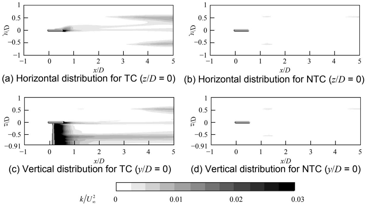
Fig.11 Contour plots of turbulence kinetic energy (horizontal and vertical cross-sections through the rotor center)
