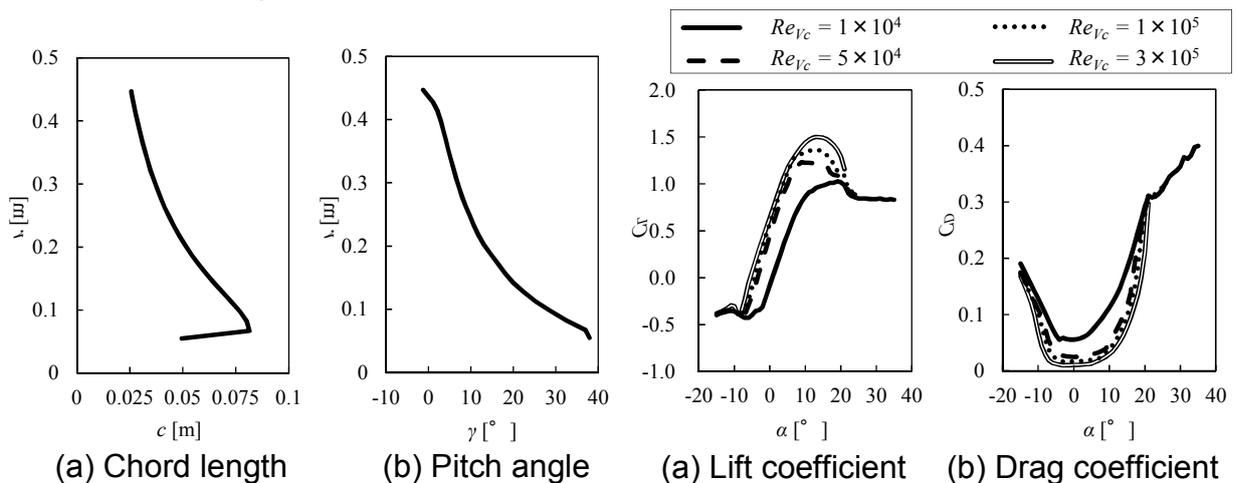
Fig.4 Distribution of the blade chord length and pitch angle as a function of the radial position.
