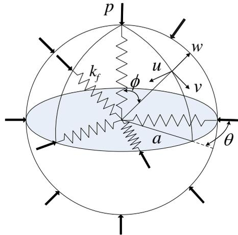
Fig.1 Hydrostatically pressurized spherical shell filled with an elastic medium
