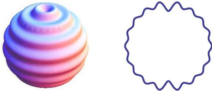
Fig.3 Buckling modes with  $a/h = 50$  and  $ak_f/E = 0$
