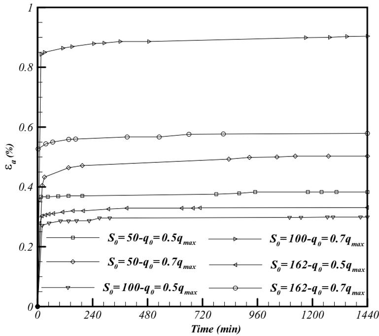
Fig. 3 Instantaneous and delayed axial strains of specimens before wetting phase.
