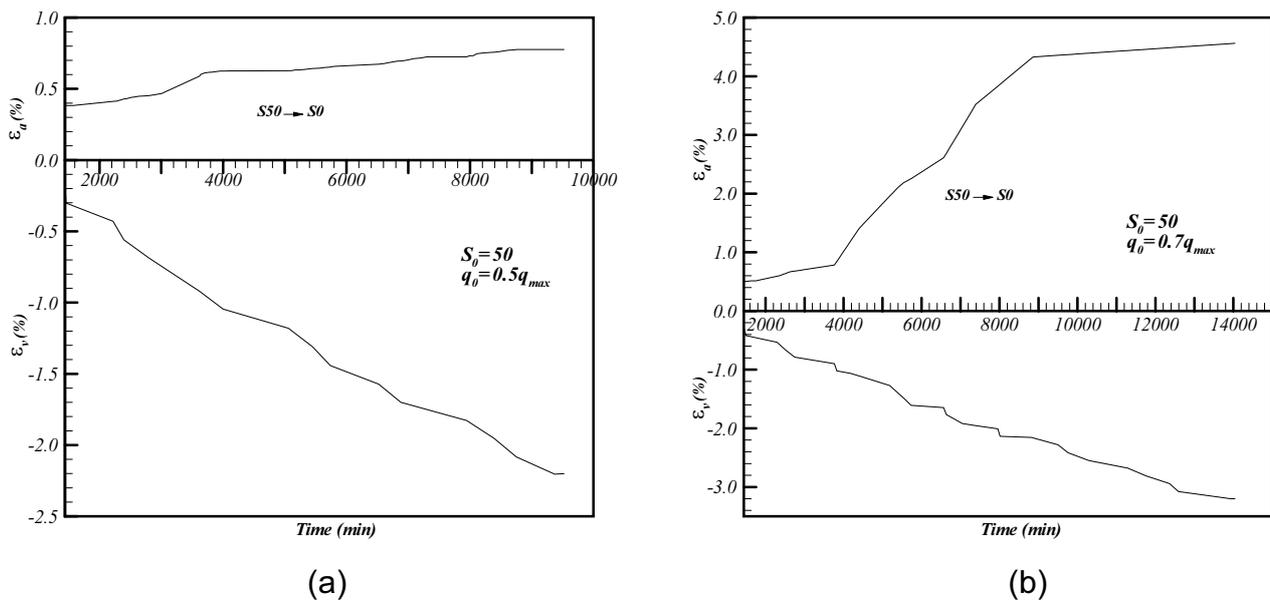
Fig. 4 Axial and volumetric strains of specimen during wetting phase with initial suction of 50 kPa.
