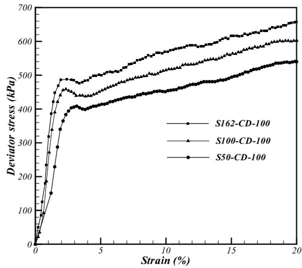
Fig. 2 Stress- strain curves of triaxial tests for different initial matric suctions
