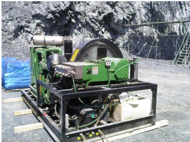
Fig. 3. A plunger type pump
