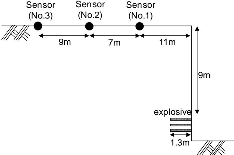
Fig. 5. Locations of vibration sensor installation (side view)
