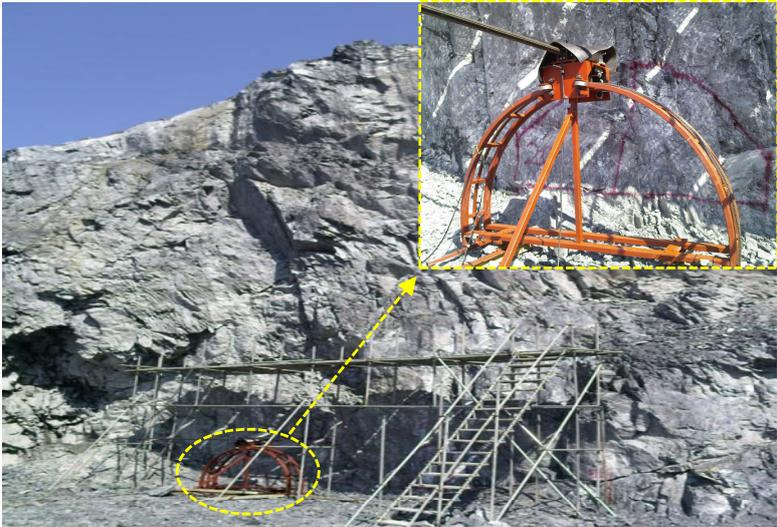
Fig. 4. Abrasive waterjet system setup
