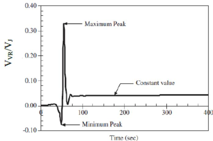
Fig. 8 Typical time history of the vertical/axial velocity (Shehata and El Damatty, 2007)
