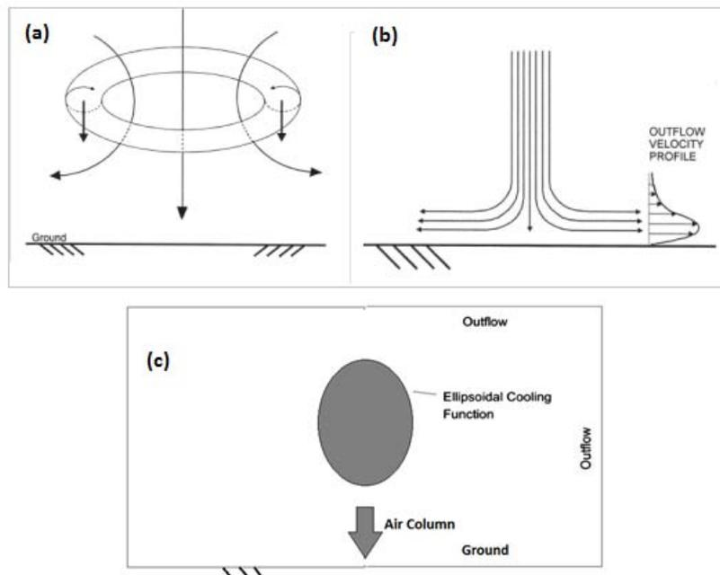
Fig. 2 a) Vortex Ring Model, b) Impinging Jet Model and c) Cooling Source Model (diagrams are from Savory *et al.* (2001b) and modified from Vermeire *et al.* 2011)
