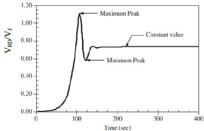
Fig. 7 Typical time history of the horizontal/radial velocity (Shehata and El Damatty, 2007)
