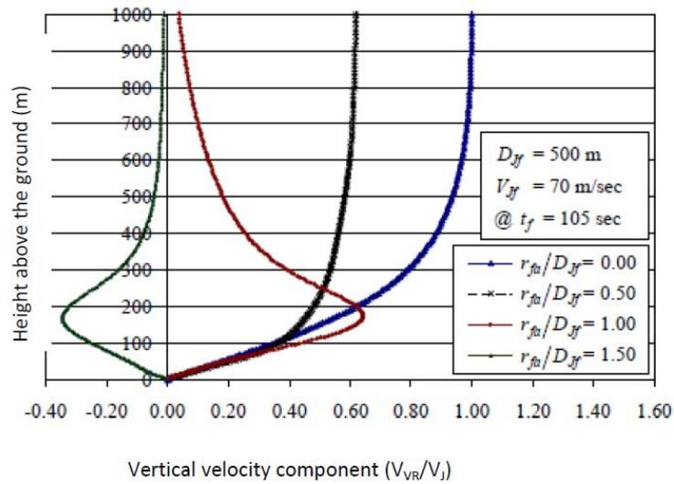
Fig. 5 Vertical profile of the vertical/axial outflow wind speed (Shehata *et al.*, 2005)
