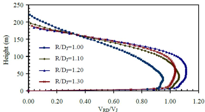
Fig. 4 Vertical profile of the horizontal/radial outflow wind speed (Shehata *et al.*, 2005)
