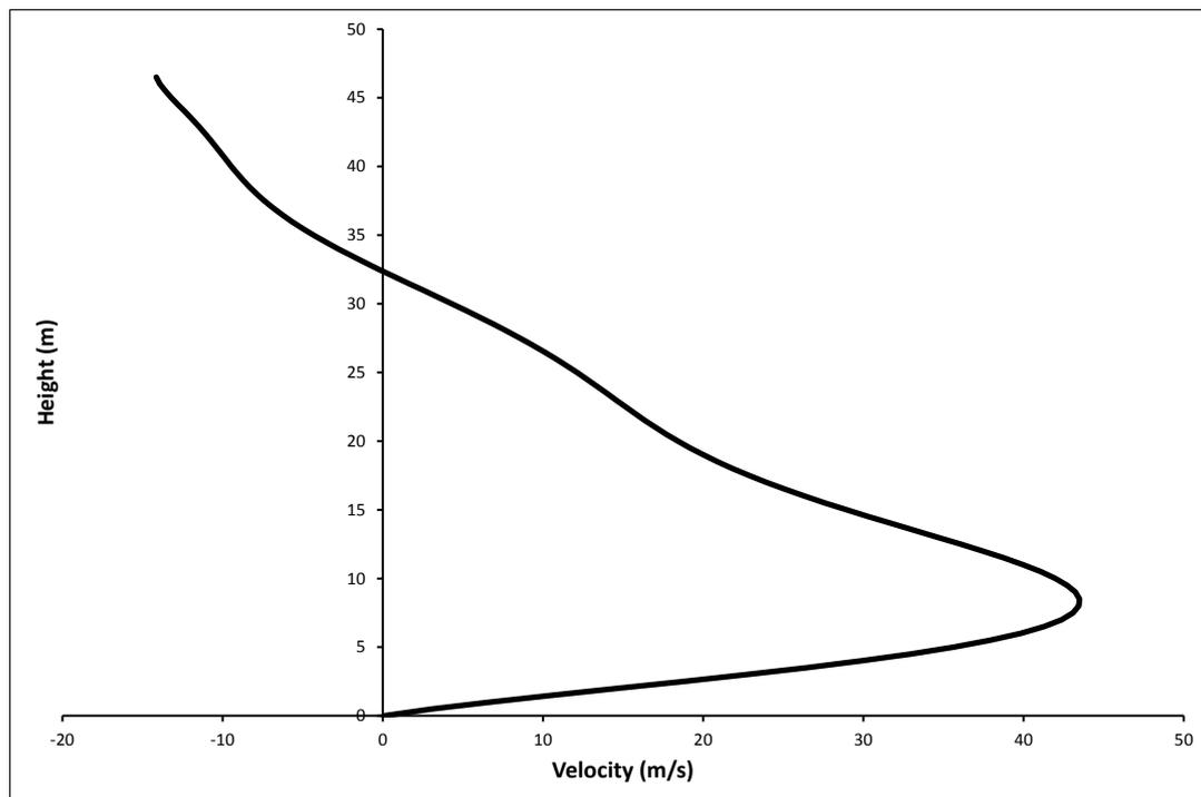
Fig. 17: Velocity profile along transmission tower height – X (transverse) direction
