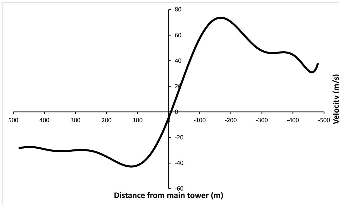
Fig. 20: Transverse velocity profile along the transmission lines
