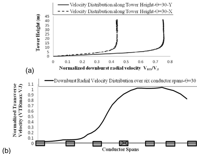
Fig. 14 (a)  $V_{RD}$  distribution along tower height with  $\theta = 30^\circ$ ,  $R/D_J = 1.6$  and  $D_J = 500$  m and (b)  $V_{RD}$  distribution over six line spans with  $\theta = 30^\circ$ ,  $R/D_J = 1.6$  and  $D_J = 500$  m (El Damatty *et al.*, 2013)
