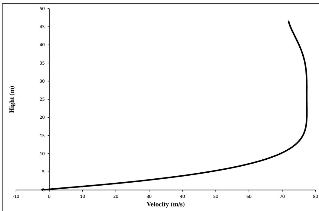
Fig. 18: Velocity profile along transmission tower height – Y (longitudinal) direction
