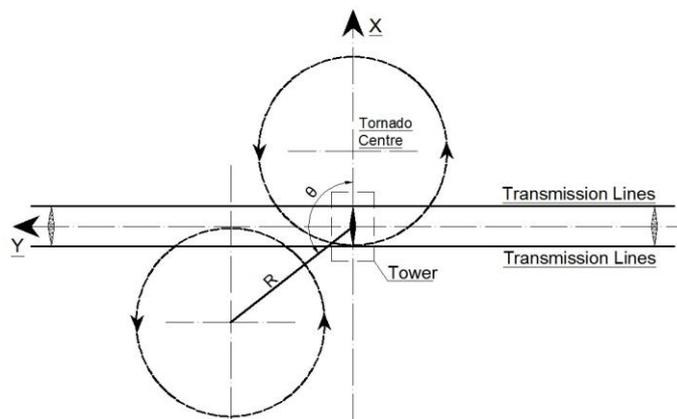
Fig. 16: Tornado configuration relative to a transmission line system
