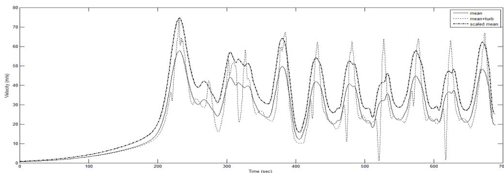
Fig. 9: Contribution of the turbulent component to the overall wind velocity
