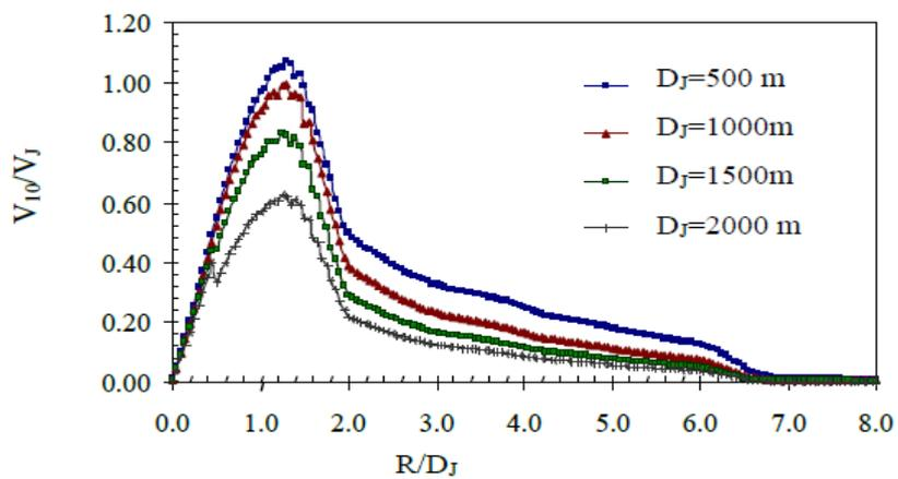
Fig. 6 Downburst reference horizontal velocity ( $V_{10}$ ) at 10 m height. (Shehata *et al.*, 2005)
