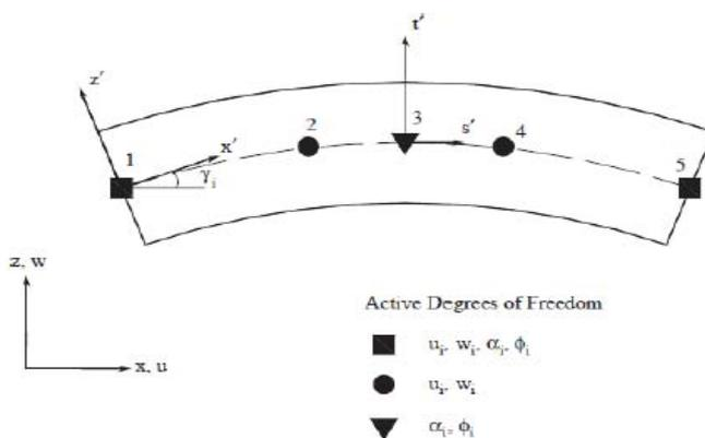
Fig. 10 Consistent beam element coordinate systems and degrees of freedom (Gerges and El-Damatty, 2002)
