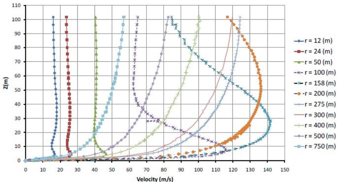
Fig. 15 Vertical profile of tangential component for different radial distances from F4 tornado centre
