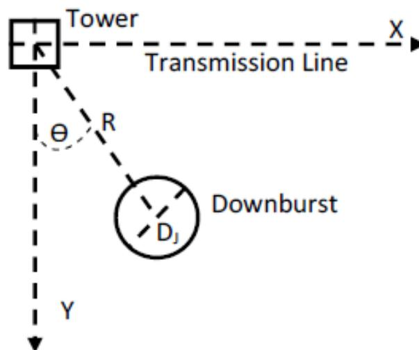
Fig. 3 Downburst parameters with respect to the tower of interest
