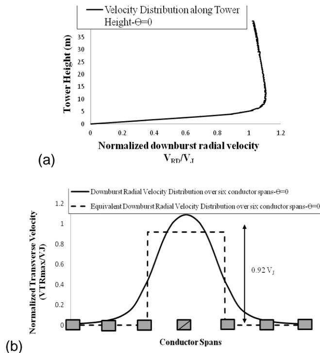
Fig. 13 (a)  $V_{RD}$  distribution along tower height with  $\Theta = 90^\circ$  and  $0^\circ$ ,  $R/D_J = 1.2$  and  $D_J = 1000$  m and (b)  $V_{RD}$  distribution over six line spans with  $\Theta = 0^\circ$ ,  $R/D_J = 1.2$  and  $D_J = 1000$  m (El Damatty *et al.*, 2013)
