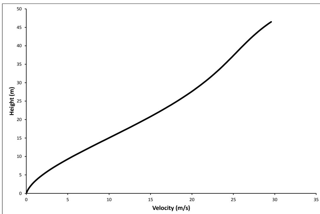
Fig. 19: Velocity profile along transmission tower height – Z (vertical) direction
