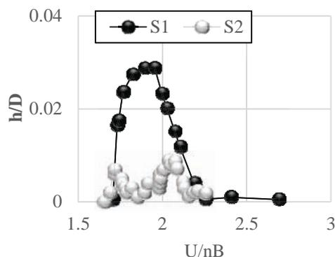
Fig. 5 V-A curves of each deck in single disposition
