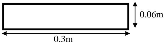
Fig. 3 Cross Section of B/D=5 model
