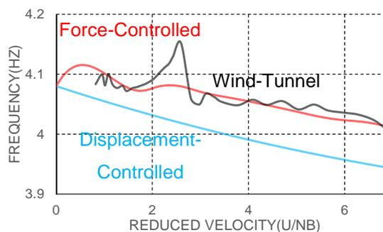
Fig.6 Aerodynamic Frequency of B/D=5
