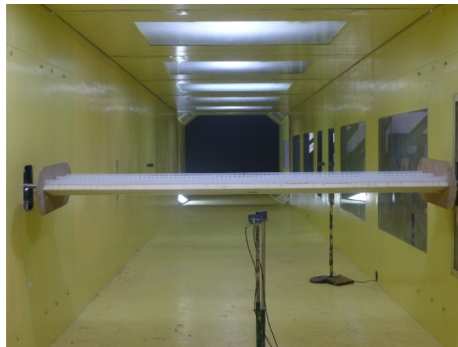
Fig. 6 The sectional model of wind-tunnel test
