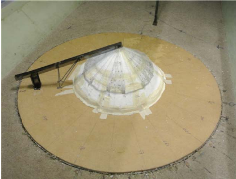
Fig. 2 1/100 scale pressure-tapped wind-tunnel model of a mineral ore stockpile cover (Structure B)
