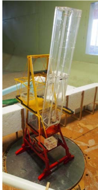
Fig. 5 1/100 scale wind-tunnel model of a shiploader (Structure C)
