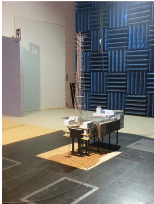
Fig. 7 1/70 scale aeroelastic model test for a flare tower (Structure D)
