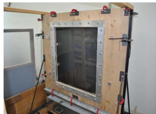
Fig.4 Pressure Box with window specimen
