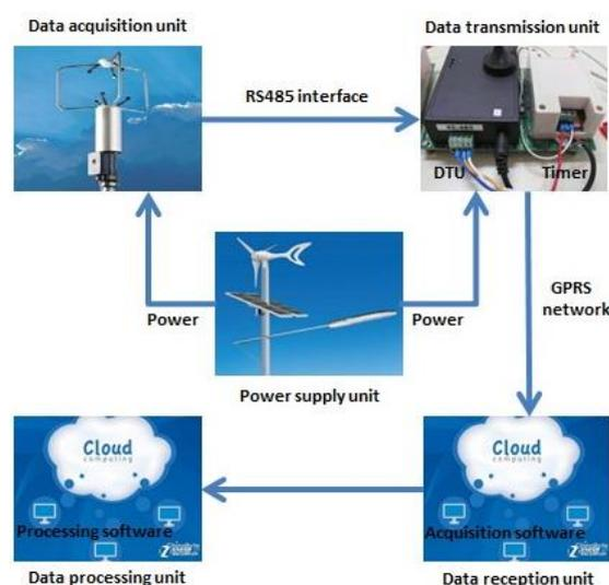
Fig. 1 Architecture of instrumentation system
