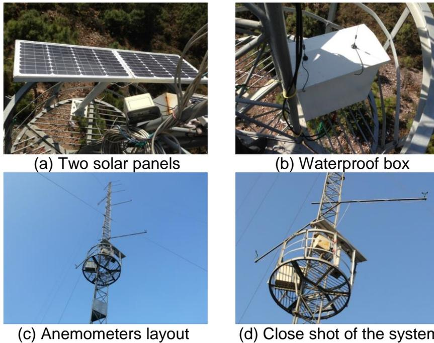
**Fig. 4** Field installation of the whole system
