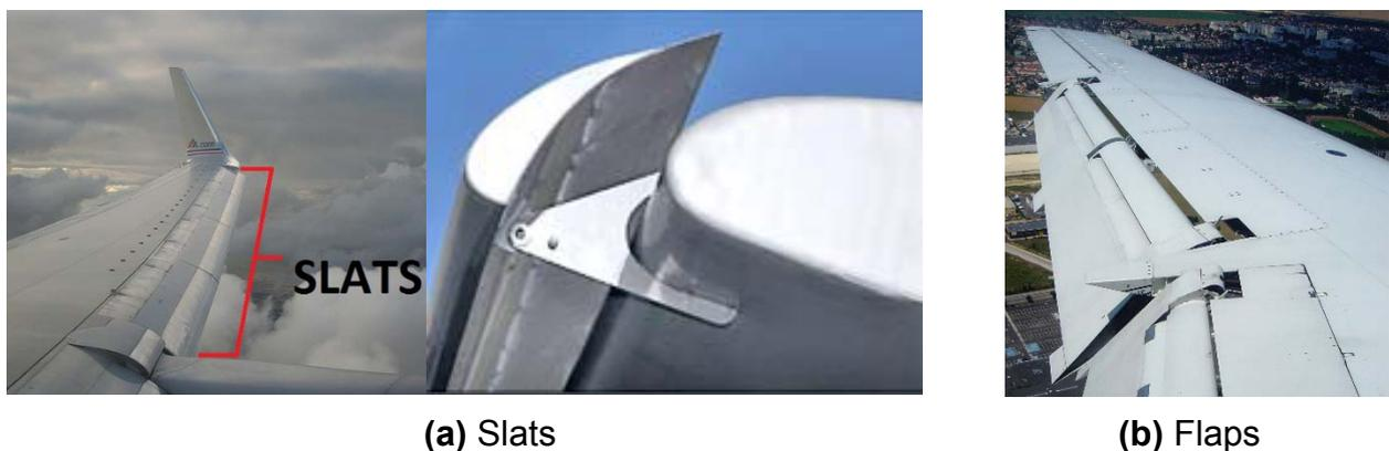
Fig. 1 Similar to an airplane landing mechanism, aerodynamic features are inspired to reduce wind loads on buildings
