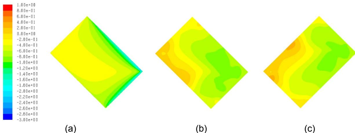
Fig. 7 Effect of the mitigation device on the mean pressure distribution on a flat roof: (a) bare roof; (b) slope-in; and (c) airfoil.
