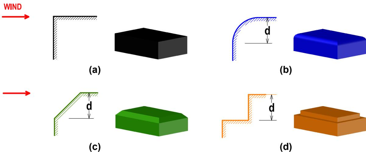
Fig. 3 Corner adjustment: (a) sharp; (b) rounded; (c) chamfered and (d) recessed corners. For each case, three different values for the dimension  $d$  were used to represent small, medium and large modifications to the corners. This created ten different testing models of flat roofs.
