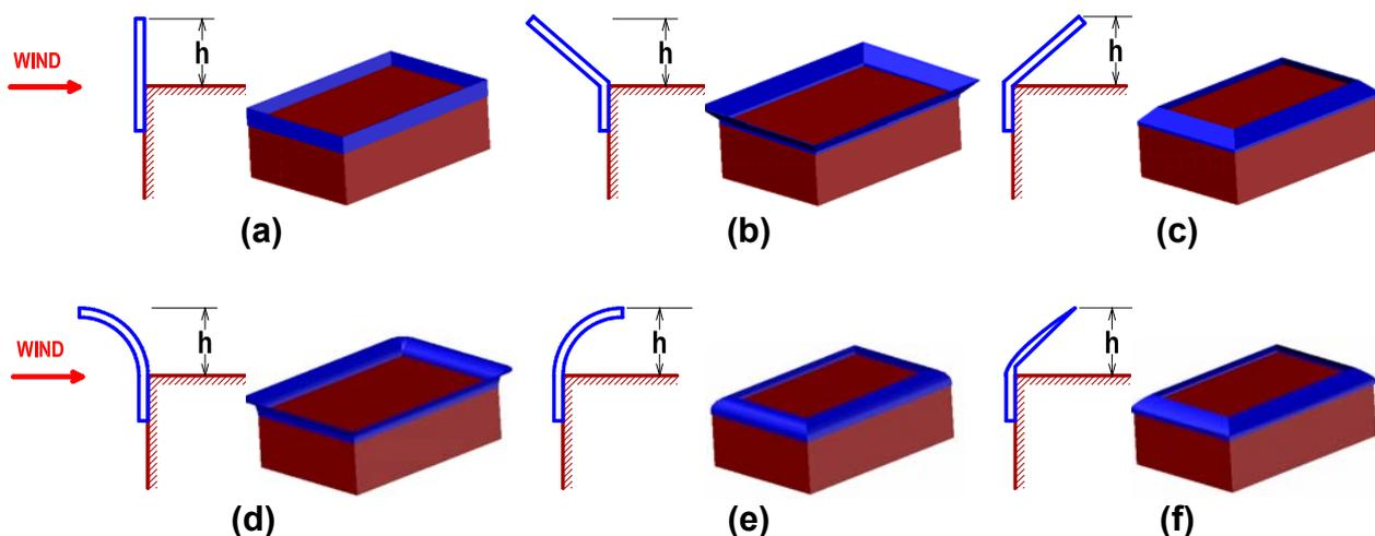
Fig. 5 Roof mitigation devices: (a) barrier; (b) barrier with an outer slope (slope-out); (c) barrier with an inner slope (slope-in); (d) circular device concaved out; (e) circular device concaved in; and (f) airfoil (half).
