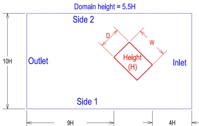
Fig. 2 Computational domain around a building under a wind direction angle of 45°. The building height H was used as a parameter for setting the dimensions of the domain.
