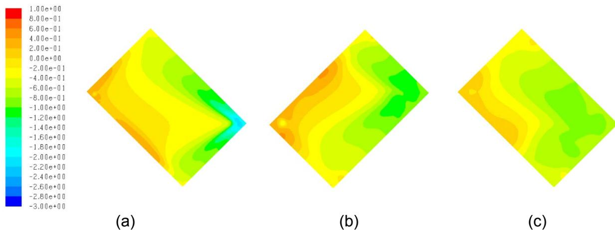
Fig. 6 Mean pressure distribution on a roof with a slope-in mitigation device: (a) small; (b) medium; and (c) large.
