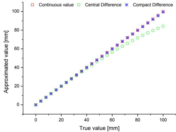
**Fig. 2** Simple Fourier error according to discretization method
