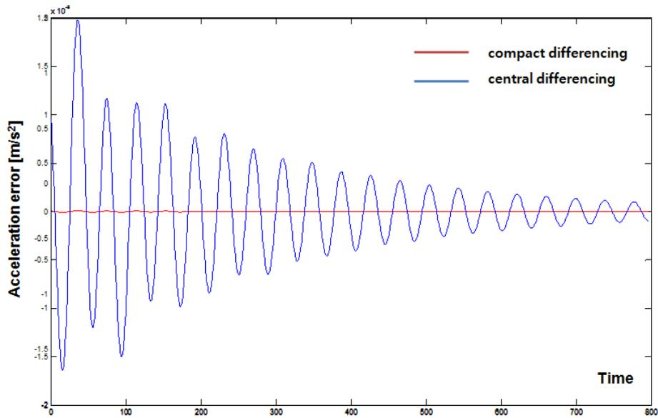
**Fig. 3** Velocity and acceleration error according to discretization method
