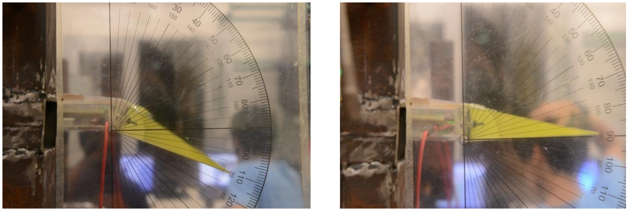
Fig. 5 Successful demonstration of the SMA-actuated trailing edge flap lowering test under 15 m/s flow speed exhibits under 5% flapping angle inaccuracy when trailing edge flap is actuated.
