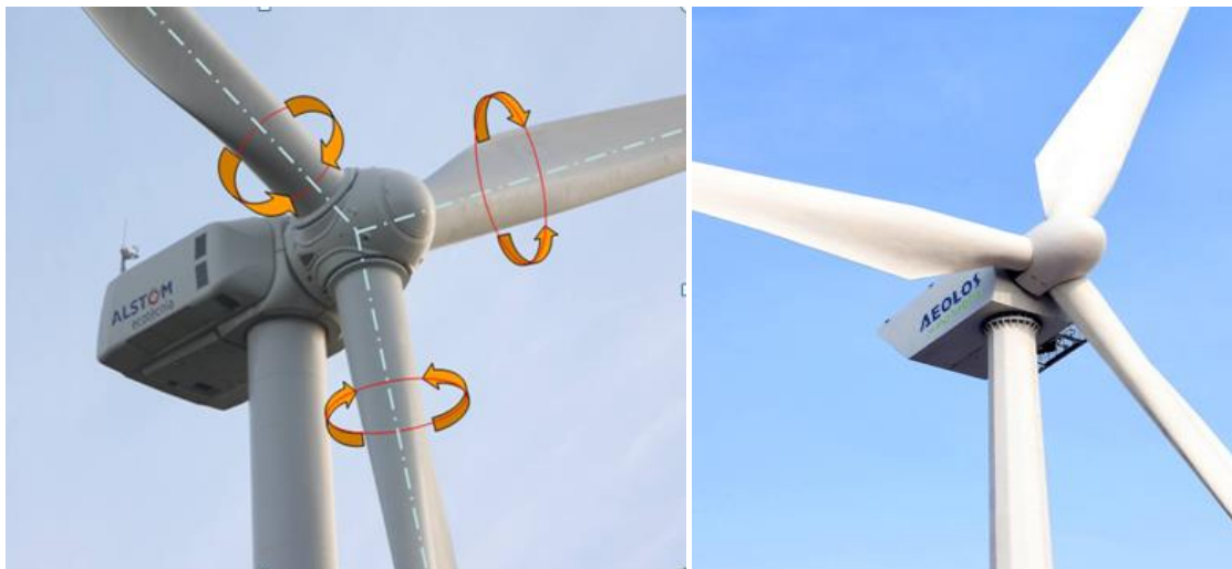
Fig. 1 [Left] Picture of a 1.25MW wind turbine rotor hub showing a circular plan form connection between the hub and the blade where the pitch control mechanism is housed. [Right] Picture of 4kW rotor hub with a simple non-movable blade-hub connection
