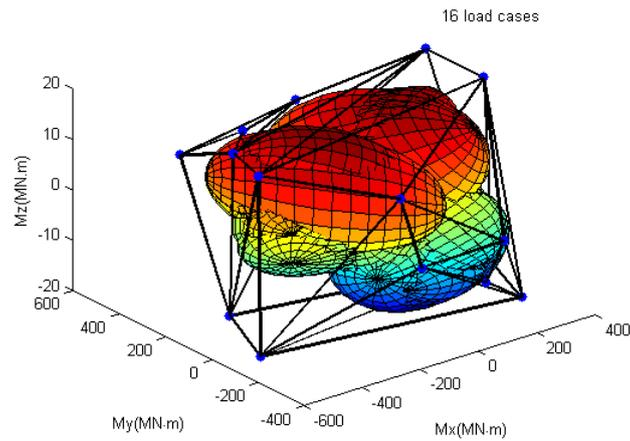
Fig. 3 Optimized design envelope with 16 load cases
