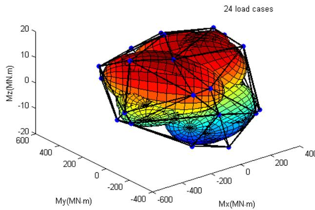
Fig. 4 Optimized design envelope with 24 load cases
