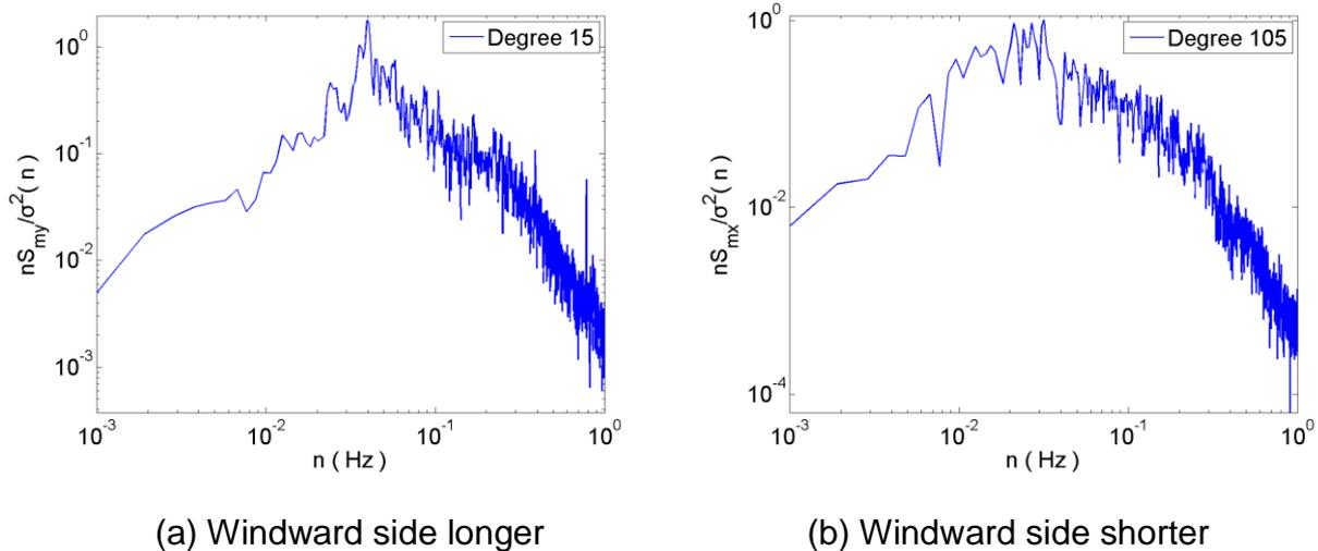
Fig. 11 Normalized PSD of across-wind base bending moment
