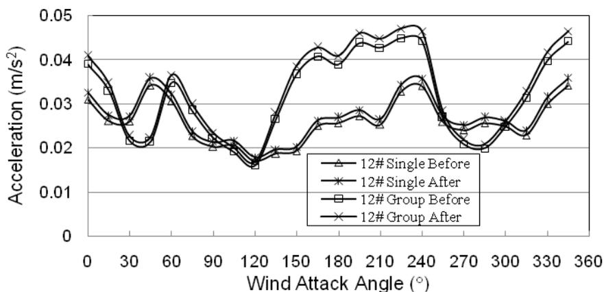
Fig. 7 Comparison of accelerations before and after mode shape correction
