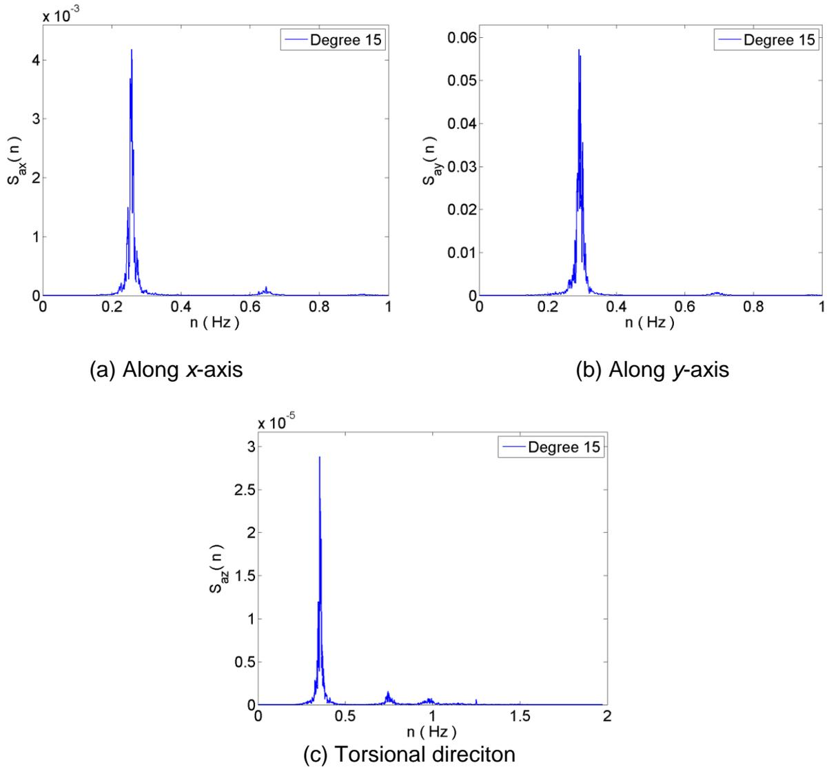
Fig.10 PSD of acceleration at 15° wind attack angle
