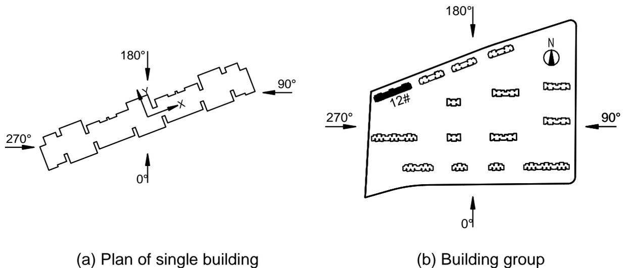
Fig. 1 Definitions of wind attack angles and coordinate system
