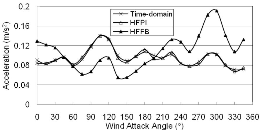
Fig. 4 Torsional acceleration responses
