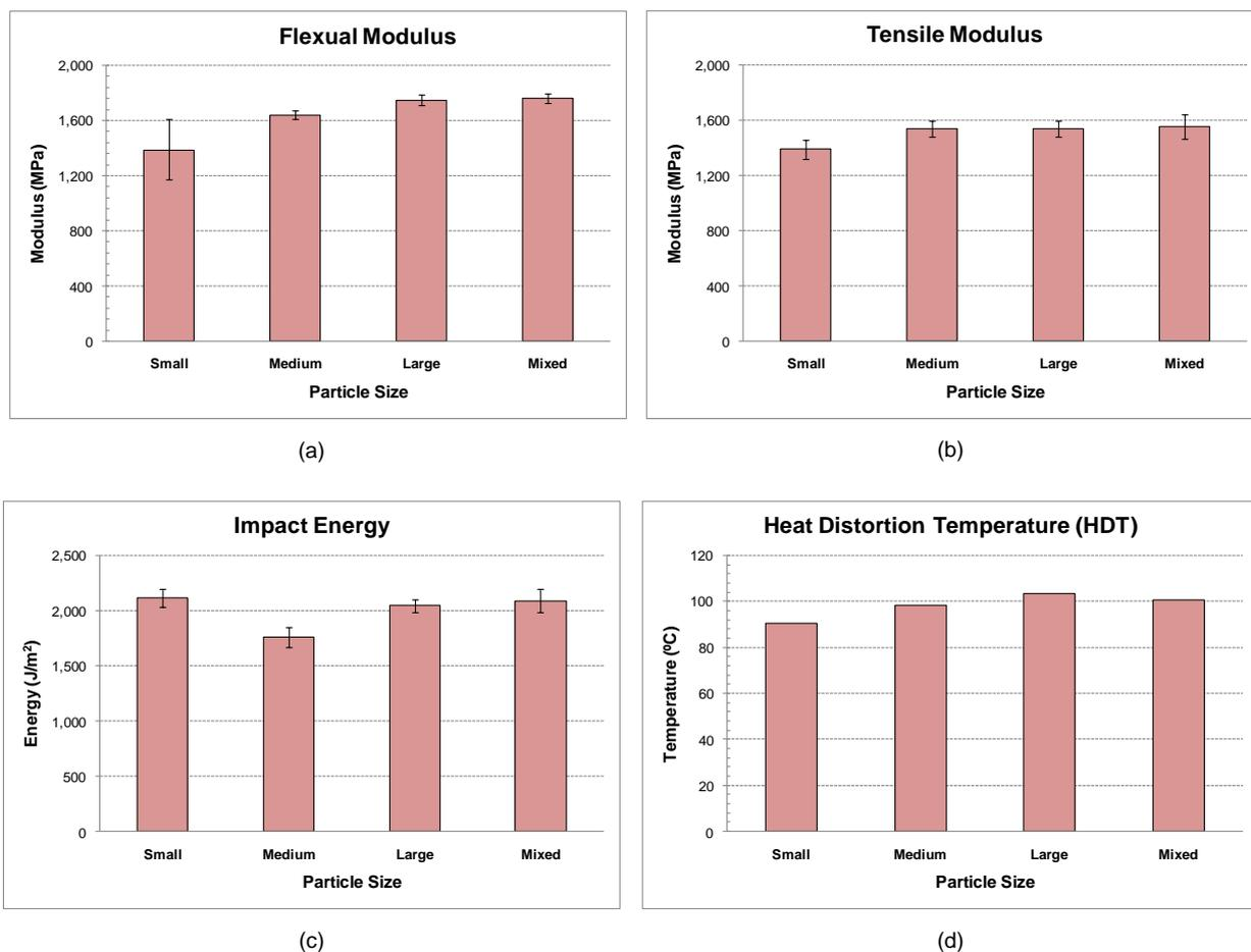
**Figure 9. Mechanical properties of WPCs prepared with 50 wt% wood and 2.5 wt% coupling agent as a function of particle size. (a) Flexural modulus (b) Tensile modulus (c) Energy required to break of the samples (d) Heat Distortion Temperature (HDT). All samples were prepared with PP matrix.**
