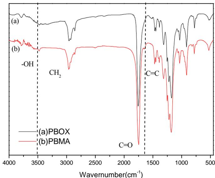
Fig. 1 FTIR spectra of (a) PBOX and (b) PBMA
