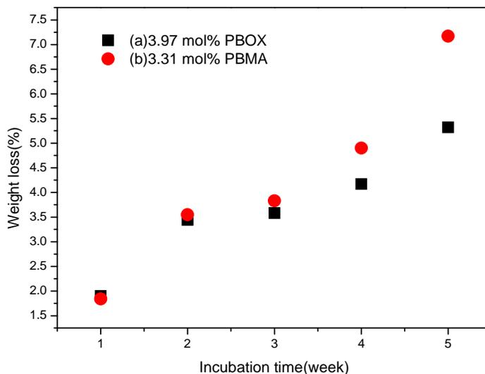
Fig. 3 The weight loss of PBOX-PU and PBMA-PU in soil degradation experiment
