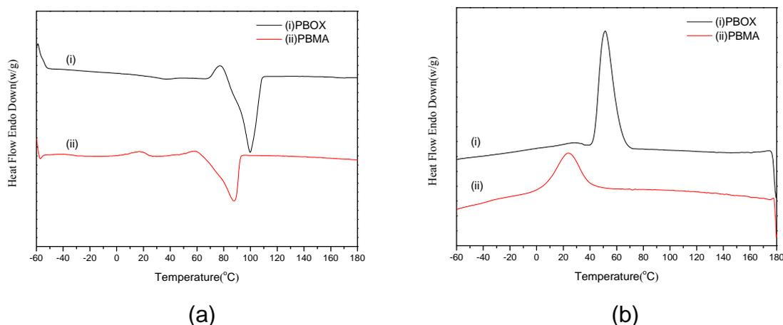
Fig. 2 DSC curves of (a) heating and (b) cooling curves of (i)PBOX and (ii)PBMA
