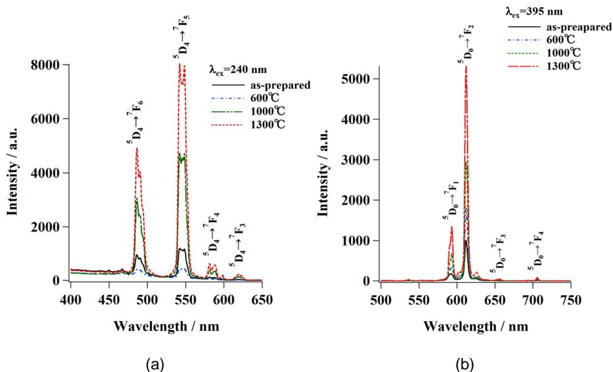
Fig. 3 Emission spectra for samples as-prepared and after heated at various temperatures for 1 h: (a)  $Y_{0.9}Tb_{0.1}NbO_4$  measured under excitation at 240 nm and (b)  $Y_{0.75}Eu_{0.25}NbO_4$  measured under excitation at 395 nm.
