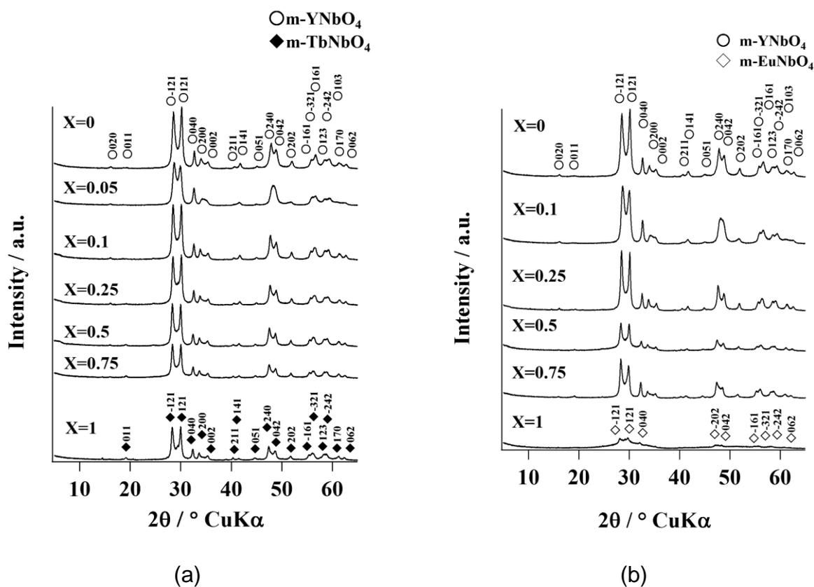
Fig. 1 X-ray diffraction patterns of precipitates obtained at various compositions of  $x=0\sim 1.0$  in (a) Y<sub>1-x</sub>Tb<sub>x</sub>NbO<sub>4</sub> and (b) Y<sub>1-x</sub>Eu<sub>x</sub>NbO<sub>4</sub> under hydrothermal conditions at 240 °C for 5 h.
