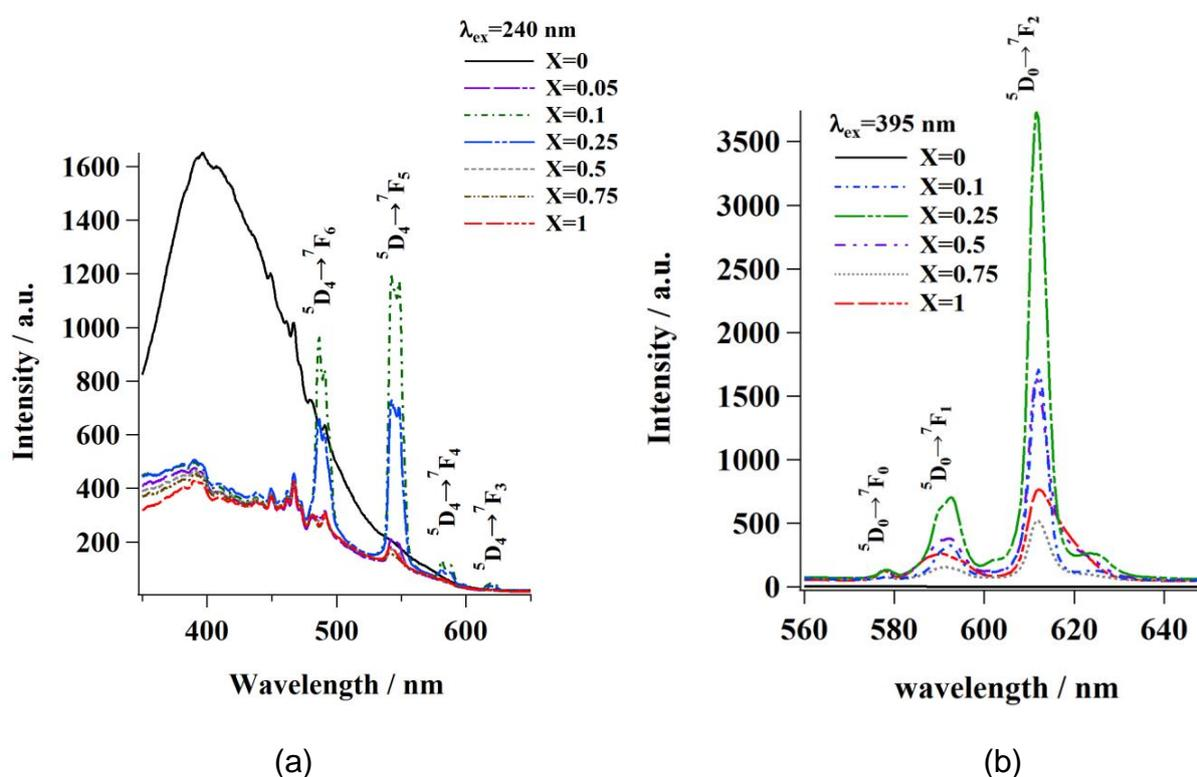
Fig. 2 Emission spectra for the as-prepared samples (a)  $\text{Y}_{1-x}\text{Tb}_x\text{NbO}_4$  measured under excitation at 240 nm and (b)  $\text{Y}_{1-x}\text{Eu}_x\text{NbO}_4$  measured under excitation at 395 nm.
