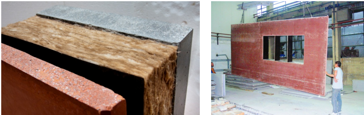
Figure 3: ECO-SANDWICH ® wall system
