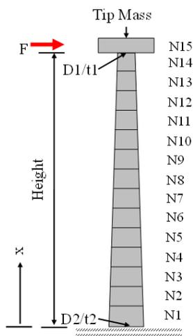
(a) 5MW wind turbine model
