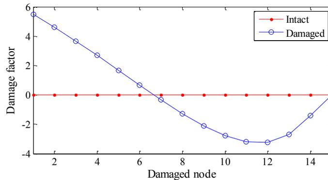
Fig. 4 Sensitivity of damage factor to 50% of damage severity
