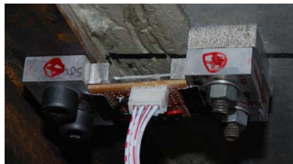
Fig. 2 A prototype of the developed relative displacement sensor
