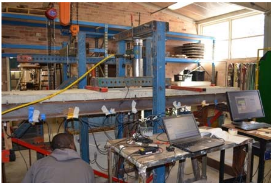
Fig. 4 Experimental setup for static loading
