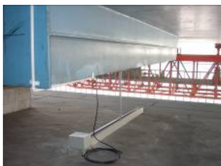
a) Displacement sensor photo at the girder end b) Temperature sensor layout Fig. 2 Temperature sensor and displacement sensor layout of the Jiangyin bridge
