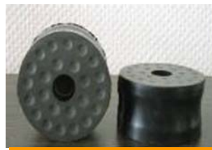
Fig. 8 High-performance slider material used in Runyang bridge
