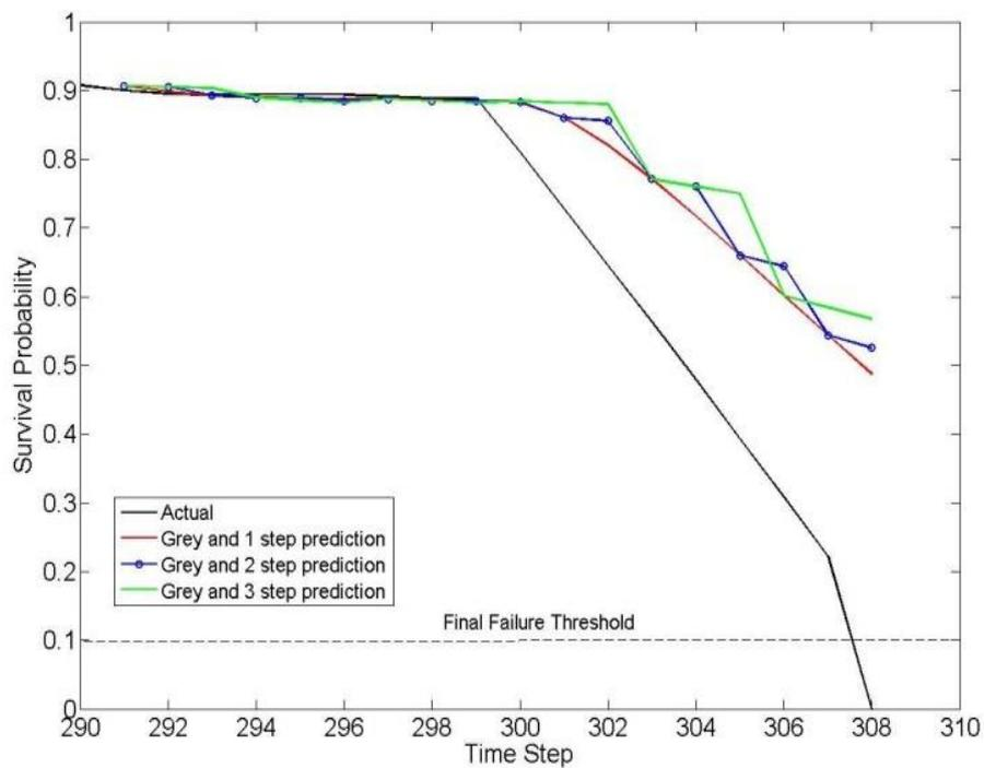
Fig.4. Grey predictions of machine's condition using one-step-ahead, two-step-ahead, and three-step-ahead techniques.
