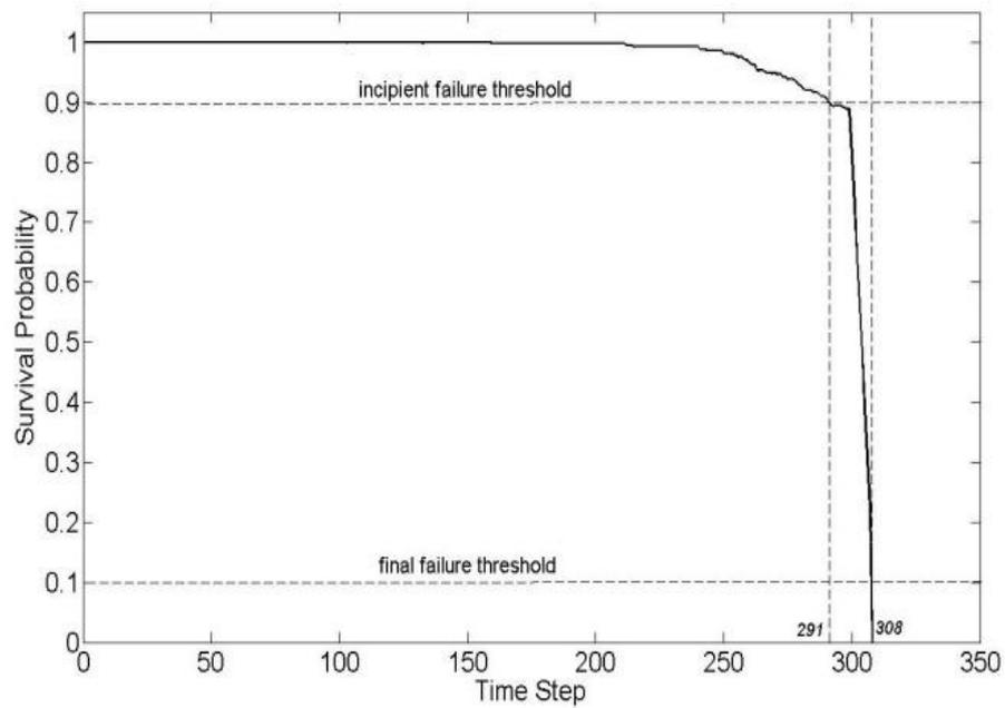
Fig.3. The degraded condition data
