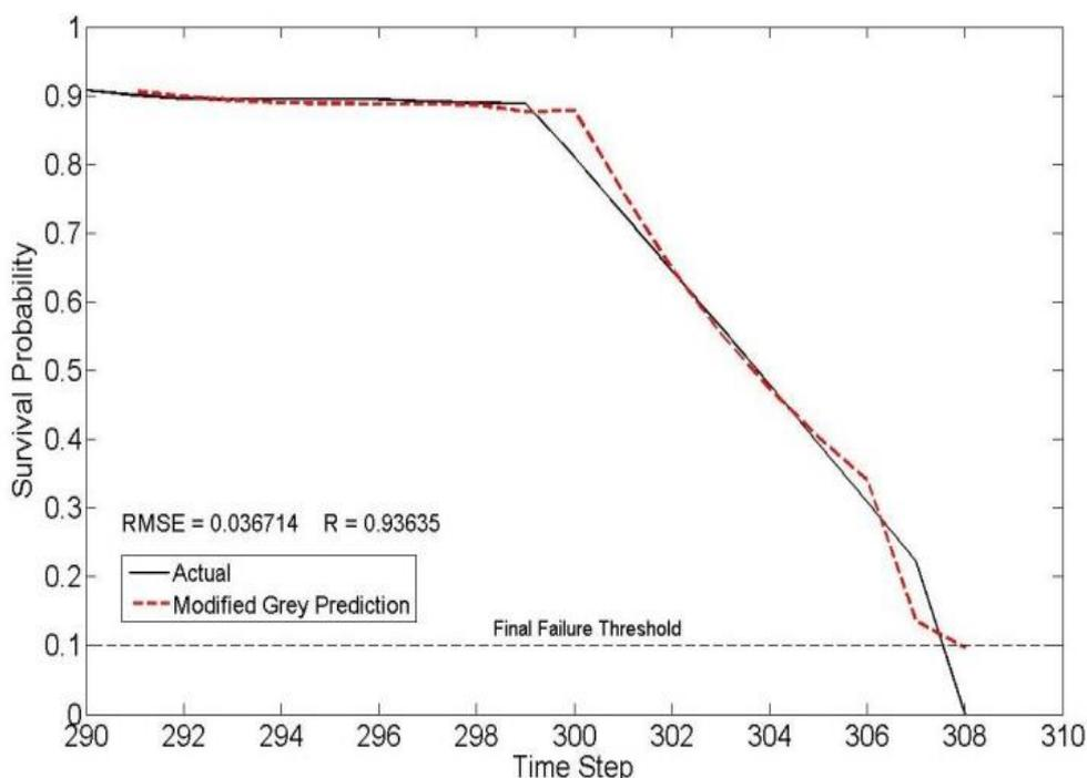
Fig.5. Modified grey prediction coupled with one-step-ahead technique.
