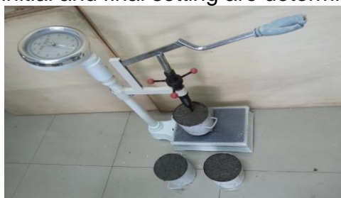
Fig. 2 Penetration resistance test
