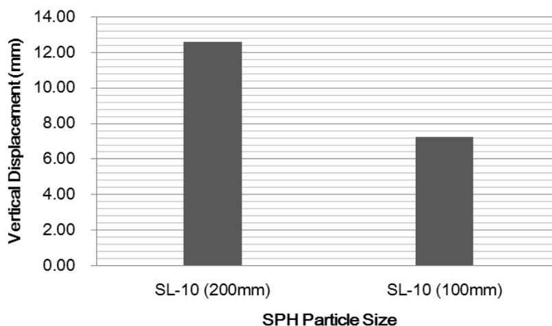
Fig. 4 Vertical displacement (mm) according to SPH particle size
