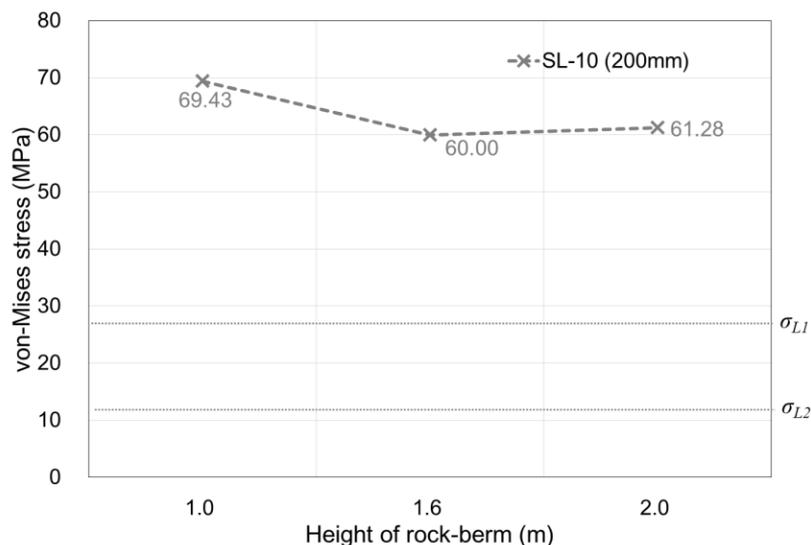
Fig. 5 von-Mises stress (MPa) according to SPH particle size and height of rock berm
