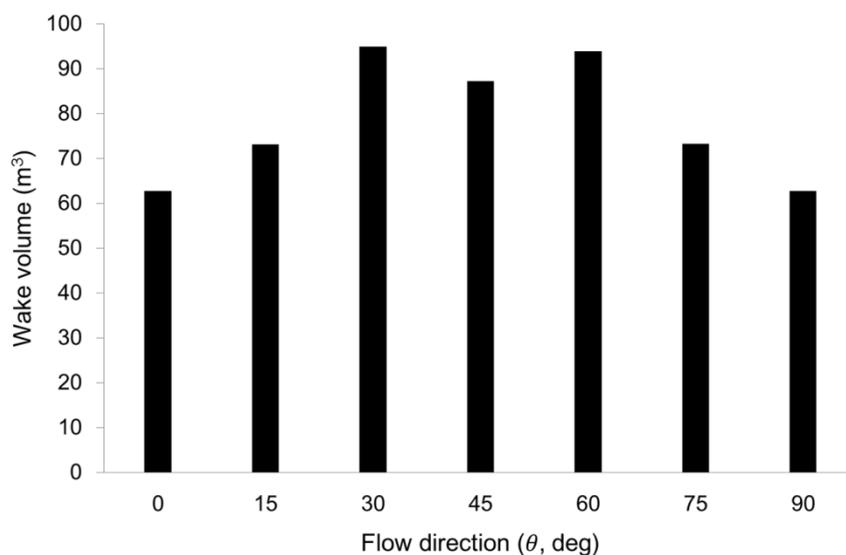
Fig. 10 Wake volumes according to flow directions (0 to 90°)
