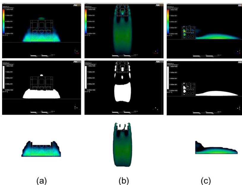
Fig. 4. Wake regions of box-type AR: (a) front view, (b) top view, and (c) side view
