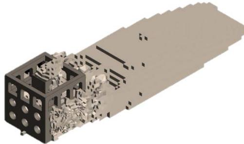
Fig. 7 Wake volume represented by summation of finite volumes, which have recirculating water flows
