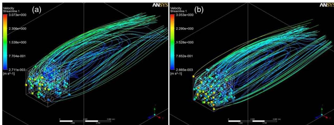
Fig. 6 Streamlines of ARs: (a) box-type AR and (b) modified AR
