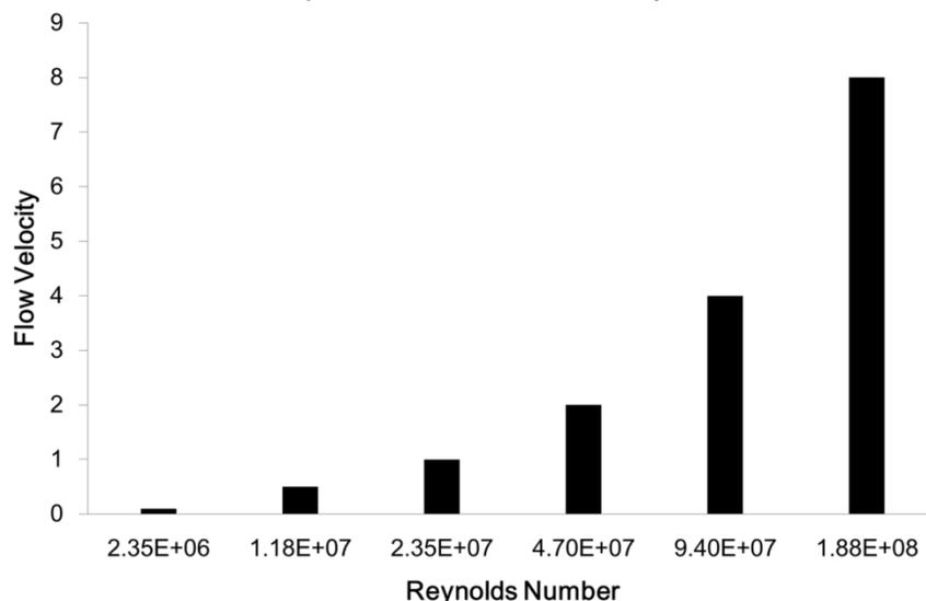
Fig. 8 Relation between Reynolds number and flow velocity
