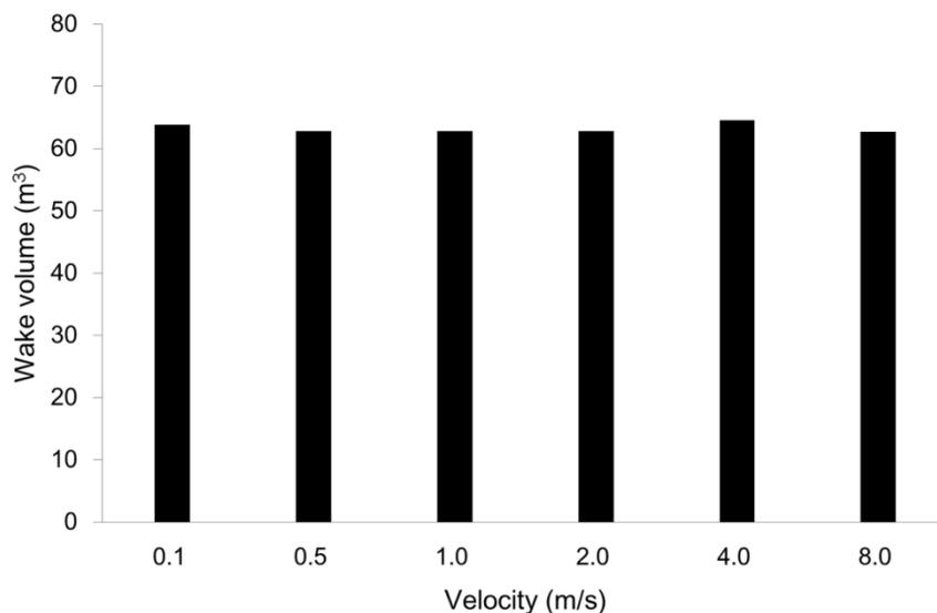
Fig. 9 Wake volumes according to inlet velocities (0.1 to 8.0 m/s)
