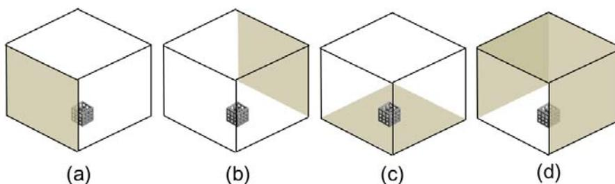
Fig. 3 Flow boundary conditions: (a) inlet, (b) outlet, (c) bottom, (d) symmetry.
