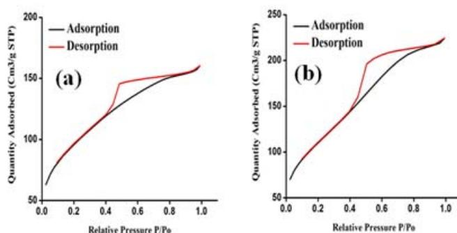
Fig.2 N2 Adsorption isotherms of (a) As-synthesized (b) after heat treatment
