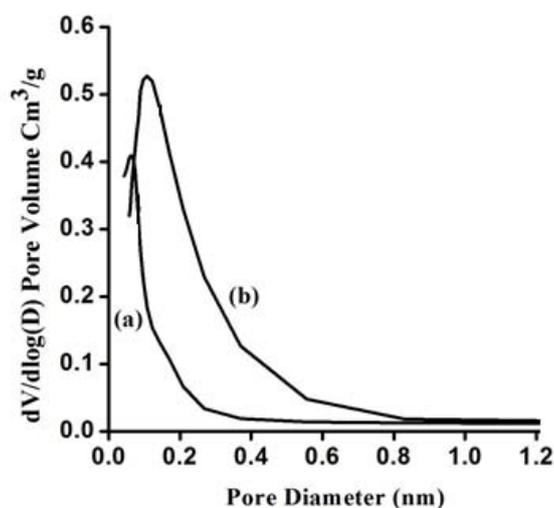
Fig.1 Shows pore size distribution curves obtained by BJH (a) As-synthesized (b) after heat treatment
