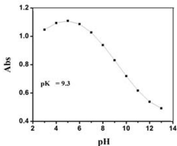
Fig. 4 pK value of encapsulated indicator hybrid sol at pH (3-13).
