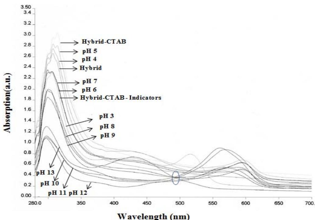
Fig.3 Absorption spectra of hybrid, hybrid-CTAB and hybrid-CTAB-indicators sol at different pH values (3-13).
