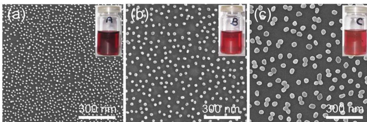
Fig.2 SEM micrographs of gold nanoparticles deposited on silica substrates: (a) smaller diameter 13 nm (colloid A), (b) medium size 25 nm (colloid B), and larger diameter particles 45 nm (colloid C). Insets show the colloidal gold solution of each sample.
