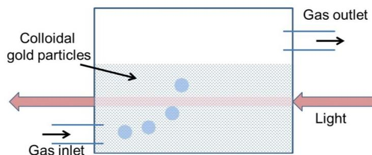
Fig.1 The set-up to produce gaseous environment for optical gas sensing of gold nanoparticles
