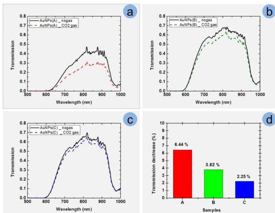
Fig.3 The experimentally measured optical transmission spectra of colloidal gold nanoparticles with and without CO<sub>2</sub> gas flow. In all three cases; (a) 13nm smaller, (b) 25nm medium, and (c) 45nm diameter larger nanoparticles, a decrease in transmission in presence of CO<sub>2</sub> gas is evident. The effect of particle size on this trend is shown in figure 3(d)
